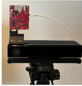
Figure 3.3 : Mmwave radar and camera. The center of the antenna array is aligned with the camera.
