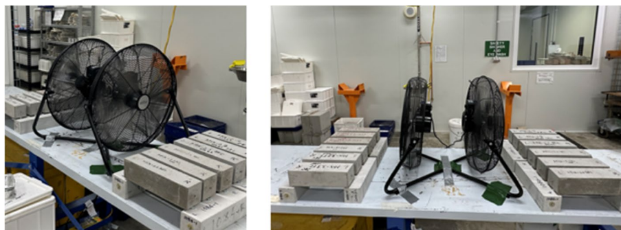
Fig. 1 38 °C and 20% R.H. controlled room including wind action
