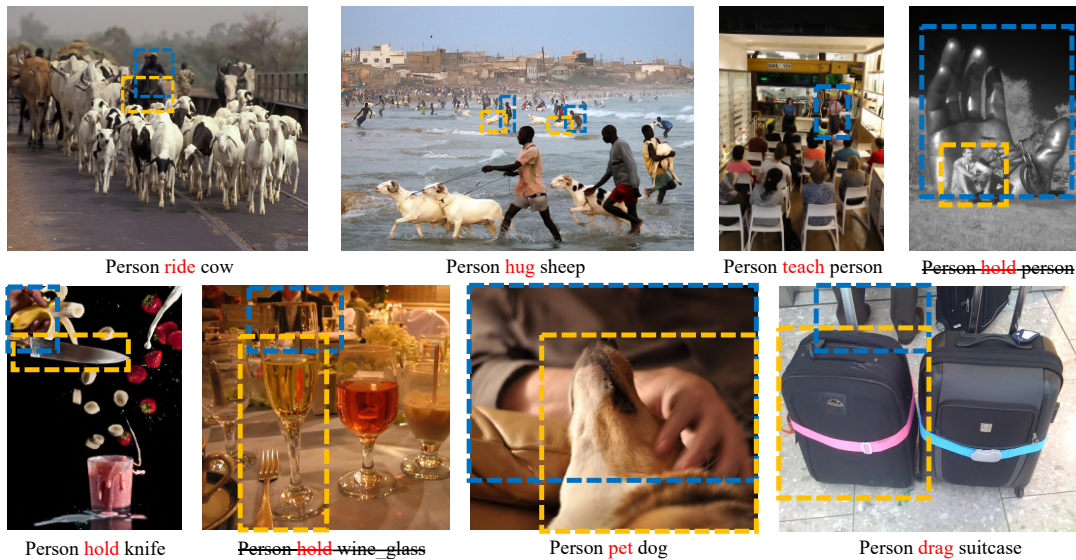
Figure 6.4 : Typical failure case on HICO-DET. Actions highlighted in red indicate missing predictions that should be detected, while text with strikethrough means wrong predictions that should be removed.
