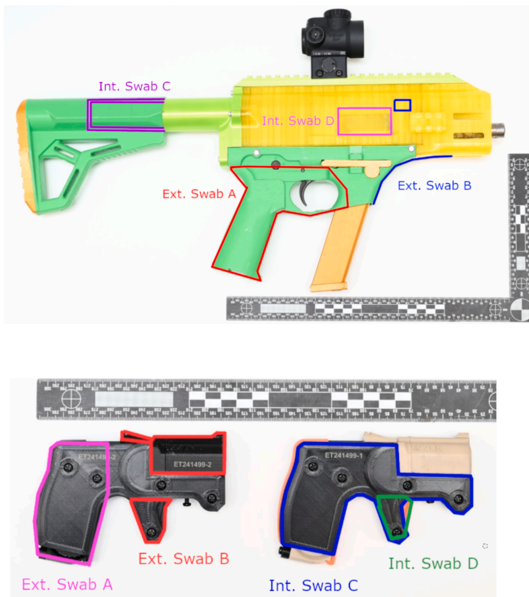
Fig. 1. FGC-9 rifles (A) and Harlot pistols (B) and the areas that were sampled for DNA from the exterior and interior surfaces.
