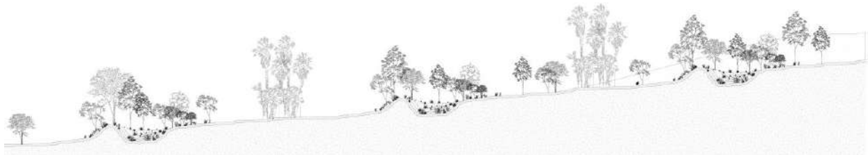
Figure 4-26: The imaginary section shows the predicted future of the site after water-harvesting techniques have been implemented. It also shows how the swales with the trees can create green and natural zones that can be used as an open space for locals and visitors to interact with nature in the future. Source: The researcher.
