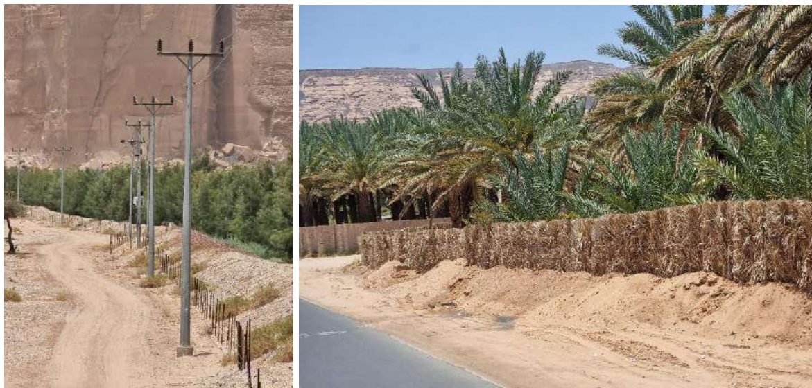
Figure 5-25: It is sometimes necessary to combine two to three techniques to enhance the protection of a site. In the left photo, locals combine the metal fence with oqoom and plant a fence to protect the oases from the flash flood. In the right photo, they combine washea with oqoom (sand berms) to support the washea . Source : Photos by the researcher and published in Alshami et al (2025).
