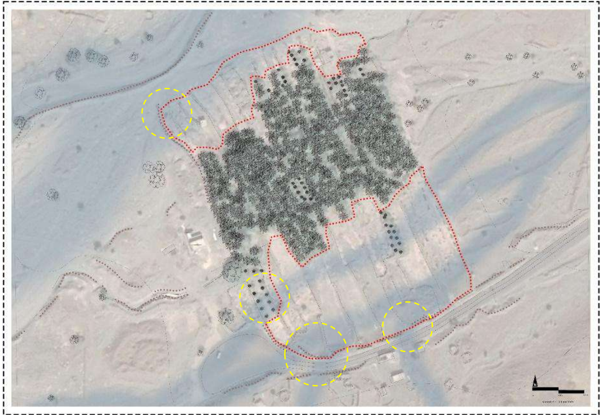
Figure 5-5: This is the VS-3 Shalal Site. The area surrounded by a red dotted line contains the degraded oases. The brown dotted lines represent the sand berms that prevent flash floods from damaging the oases and the water spring. The yellow-circled areas contain the unmaintained berms that require attention. Source: Map from Google Maps, modified by the researcher.
