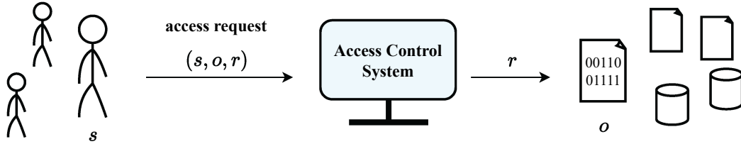
FIGURE 7.2: To exercise right r on object o , subject s sends a request (s, o, r) to the access control system.
