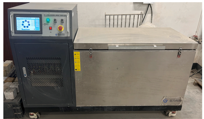
Fig. 2. HC-LSB fully automatic concrete sulfate wet-dry cycle testing machine.
