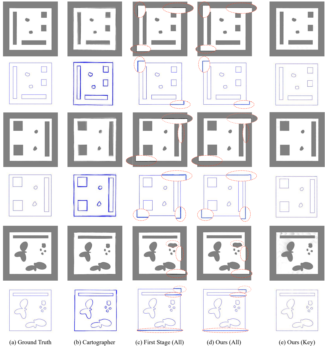
FIGURE 3.8: The OGMs and point cloud maps generated from ground truth poses and different approaches for each simulation dataset. The areas marked with red dots highlight where our method outperforms the results of the first-stage optimization alone.
