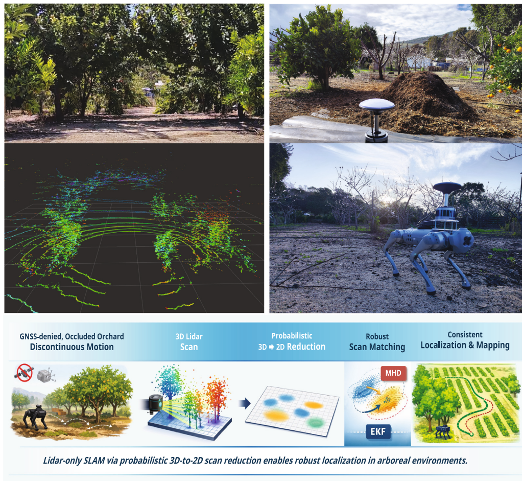
Fig. 1. Fruit orchard with dense canopies: RGB camera view in summer (top-left) and corresponding 3D lidar scan (bottom-left). The same orchard row in winter (top-right) and the legged robot with the lidar and GNSS employed in the experiments (bottom-right).
