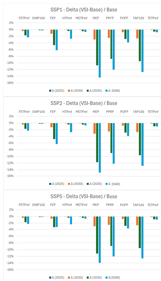
Figure 37. Relative changes in environmental impacts from VSI-aligned foreground changes, expressed as percentage change compared to the corresponding SSP-Base scenario, for the production of 1 kg of NMC111 oxide from 2025 to 2040. Relative changes in environmental impacts from VSI-aligned foreground changes, expressed as percentage change compared to the corresponding SSP-Base scenario, for the production of 1 kg of NMC111 oxide. Results are shown for each year from 2025 to 2040 and calculated as: \Delta\% = (\text{VSI} - \text{SSP-Base}) / \text{SSP-Base} \times 100 . Impact categories with no change ( \Delta\% = 0\% ) are omitted. FETPinf = freshwater ecotoxicity; FEP = freshwater eutrophication; HTPinf = human toxicity; METPinf = marine ecotoxicity; MEP = marine eutrophication; PMFP = particulate matter formation; POFP = photochemical oxidant formation; TAP100 = terrestrial acidification; TETPinf = terrestrial ecotoxicity;
