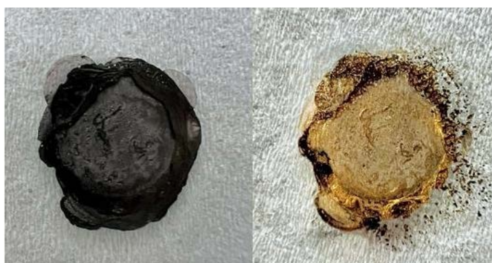
Figure 4.2 BT@AuNP ink film (left) before and (right) after exposure to a stream of ozone for 3 hours.
