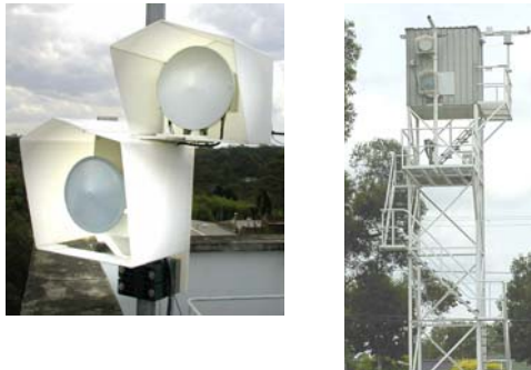
Figure 1: Millimetre wave links at the ICT Centre test bed at Marsfield. A commercial 60 GHz link (top) and an CSIRO built Gigabit link at 83 GHz.
