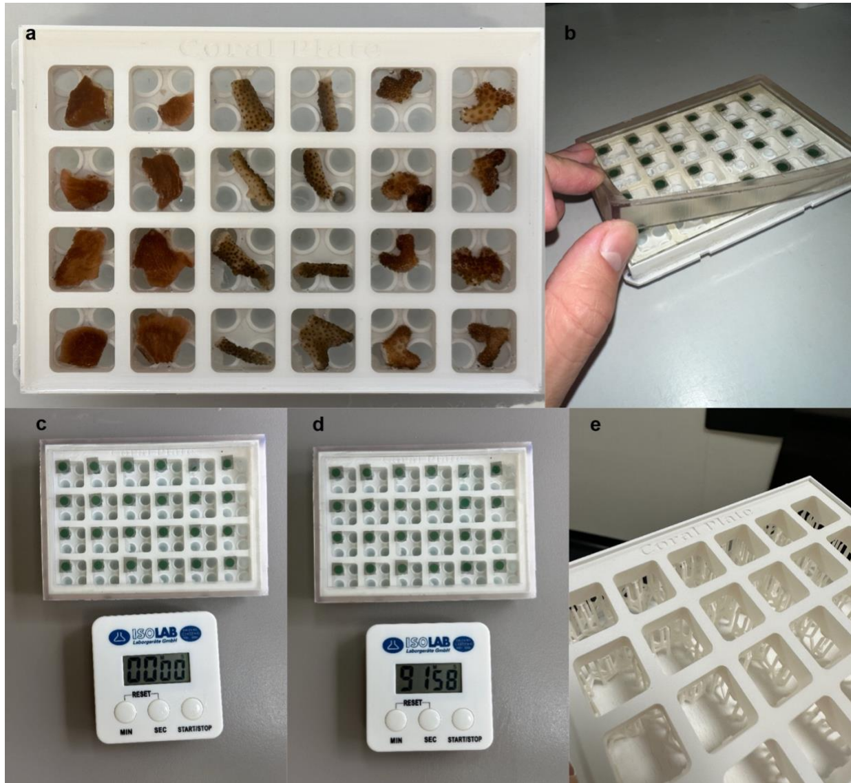
Supplementary Figure S3.1. (a) MTP adapter with coral fragment placed in each well. (b) Flexible seal ensuring the glass lid is held down and watertight conditions are maintained. (c-d) Pictures of the MTP plate filled with water and left for 90 minutes showing absence of air bubbles. (e) MTP adapter plate printed in Rigid 10K resin.
