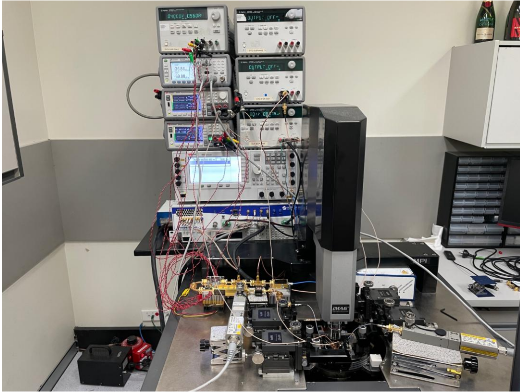
Figure 0.3: W-band driver amplifier power measurement setup.
