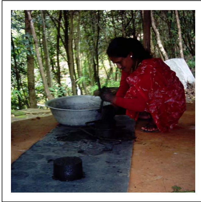
Figure 21: The manufacture of beehive briquettes in Bishankanarayan VDC
