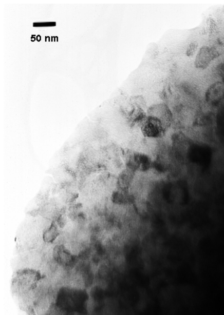
Figure 6-7: TEM image of a gel heated to 470°C for an hour.
