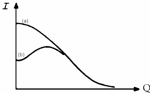
Figure 9-2: Scattering function a) of independent particles, b) with interference due to proximity of particles. Adapted from Glatter. 8
