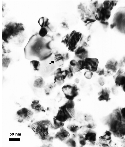
Figure 6-13: TEM image of a gel heated to 1000°C for an hour.
