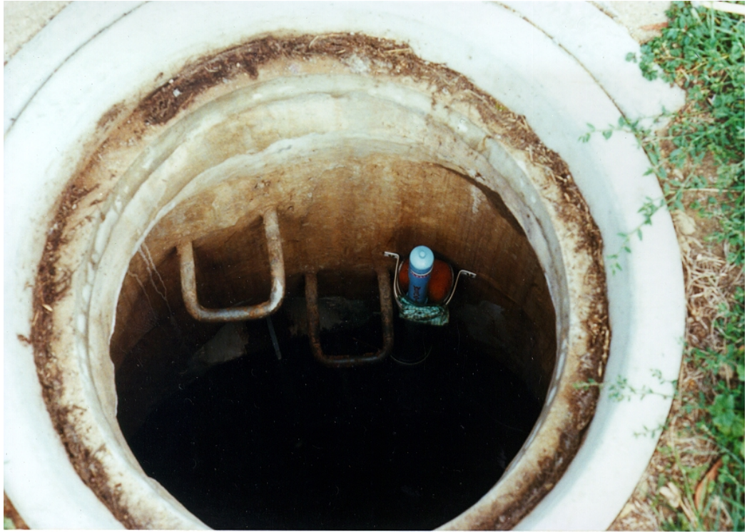
Figure 5.3.7 Looking down Manhole at 300 mm diameter Pipe Gauge
