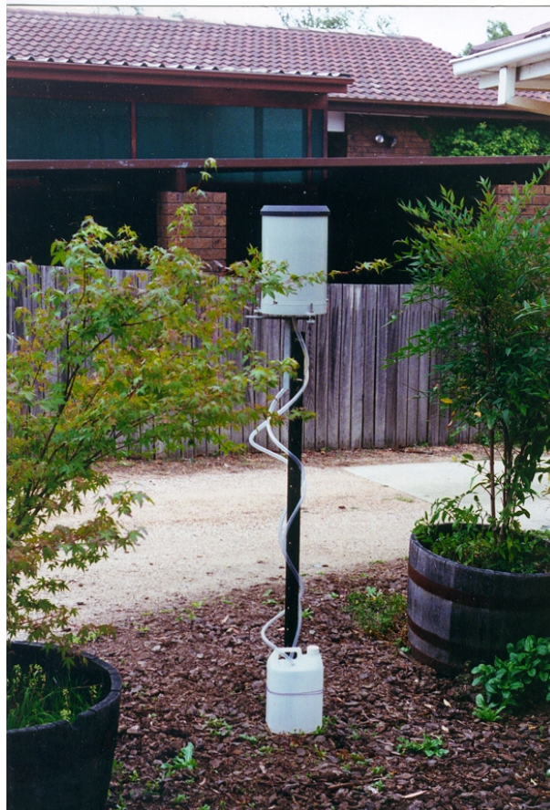
Figure 5.3.18 Spence Rainfall Pluviograph Station
