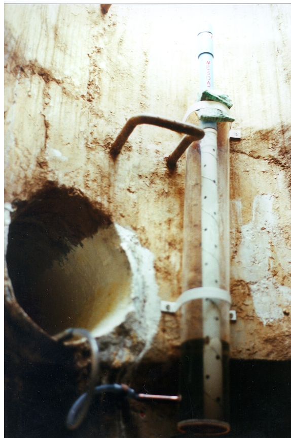
Figure 5.3.8 Close-up View of 300 mm diameter Pipe Gauge (Seen from below)
