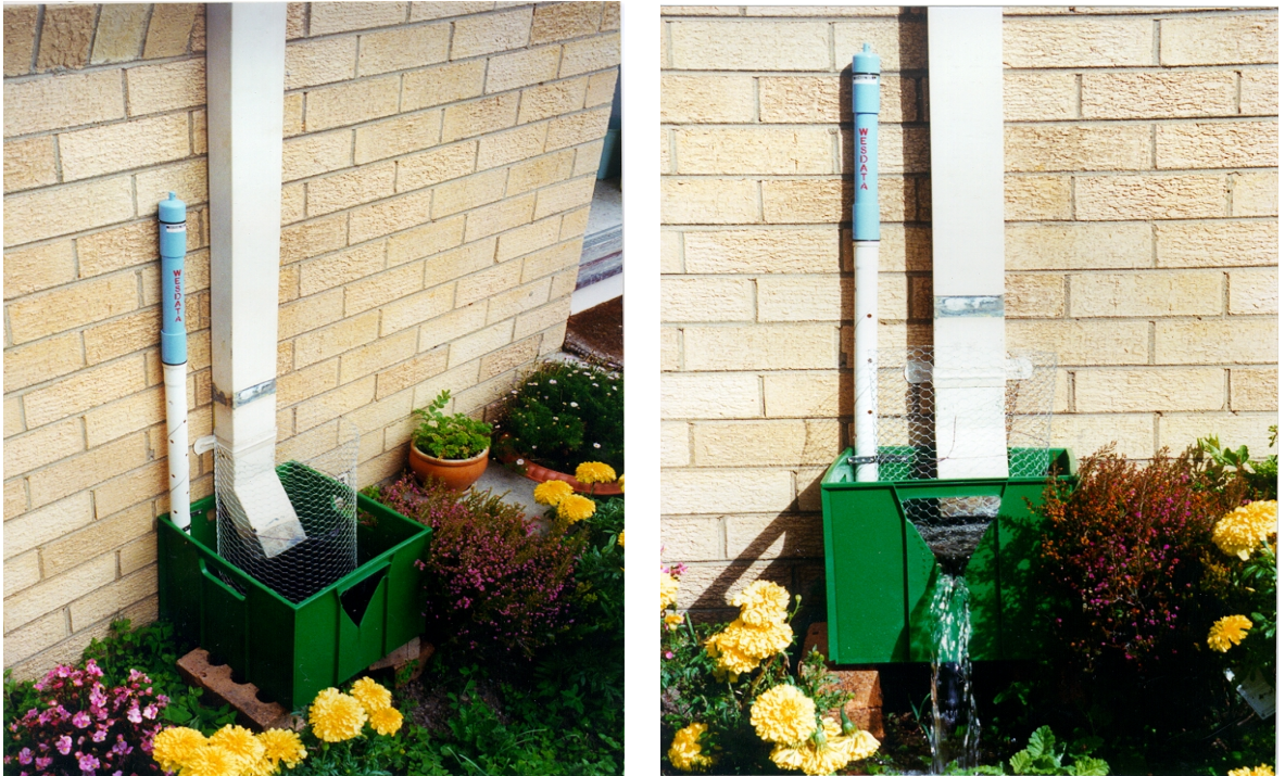
Figure 5.3.16 Close-ups of Gauging Weir and Capacitive Logger
