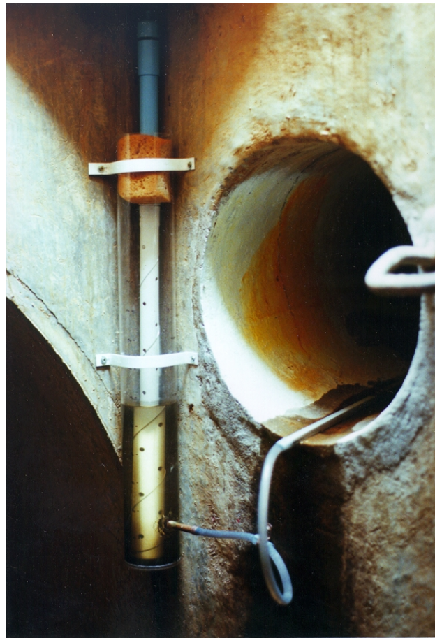
Figure 5.3.10 Close-up View of 450 mm diameter Pipe Gauge
