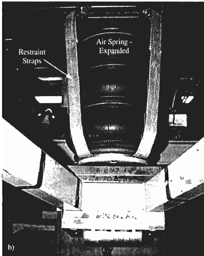
Plate 3.7: Air spring arrangement a) air spring compressed by the pendulum and b) air spring expanded and restrained by straps
