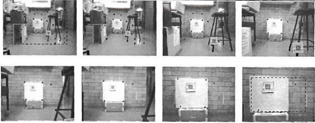
Figure 3.3: An example of a KLT tracking sequence (top left shows the set of initialised features). Notice the virtual border (dashed rectangle) within which the features are initialised and tracked. A border is required to maintain the correlation window within the image frame. A negative effect of this can be seen in the bottom right image where three of the obvious features being lost due to the border.
