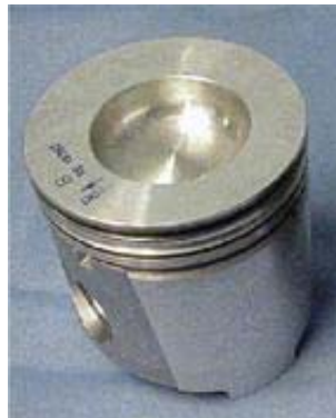
Figure 4.4: Example of an induced squish flow caused by sections of the piston coming into close proximity to the cylinder head.
