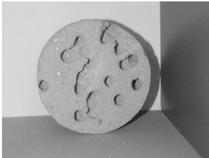
Figure 5.4 Weak Specimen showing Series of Bored Holes
