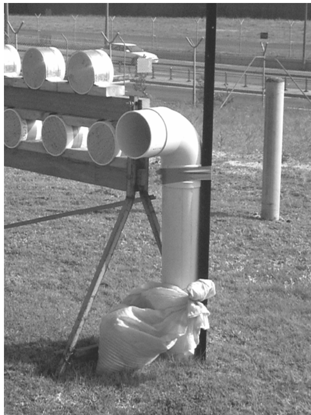
Figure 4.15 Close up view of “Periscope” Rain Collector
