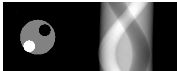
Figure 5.4: A phantom slice (left) and its corresponding sinogram (right). Each row of the sinogram is a projection of the slice at a specific view angle. The projection in the bottom row is obtained at 0^\circ and that in the top row is obtained at 180^\circ . There are 128 views (projections) equally spaced over the 180^\circ range. This simulation is noise free.
