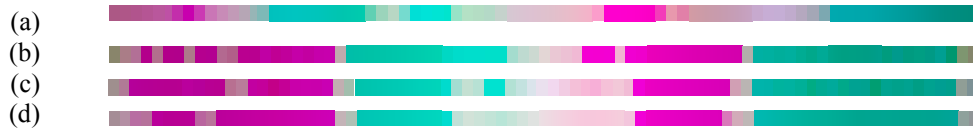
Figure 7-7. a) Measured colours in a horizontal strip through the centre of screen 10 cm from the end of the TRIMM-doped rod shown in Figure 6-8, which has been converted to RGB via calculations. b-d) modelled strip, using source diameters of 1, 2 and 3 mm, respectively.
