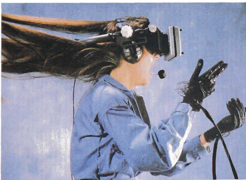
Figure 11: Heavy Technology, NASA Goggles and VPL Glove (Krueger 1991, Courtesy of W. Sisler and S.Fisher, NASA Ames Research Centre)
