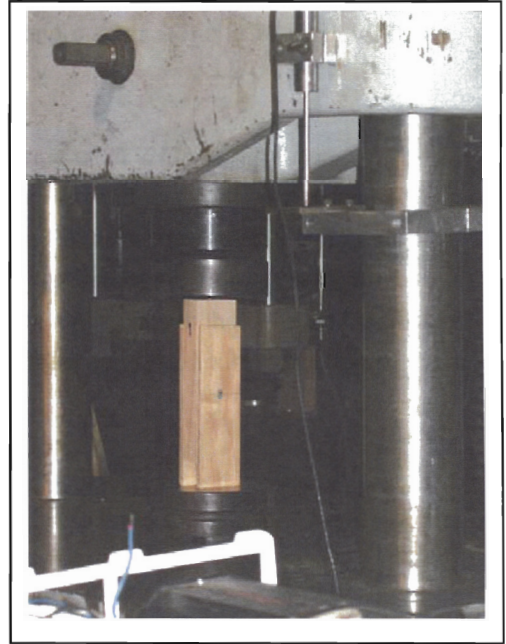
Figure 4.8 Plywood sheathing specimen for lateral nail resistance test.
