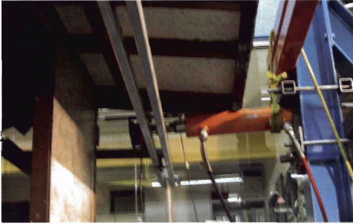
Figure 6.6 Hydraulic rams connected to the reaction frame.
