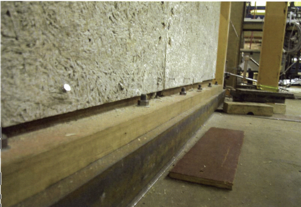
Figure 5.9 Pulling out of the nails from the timber framing.
