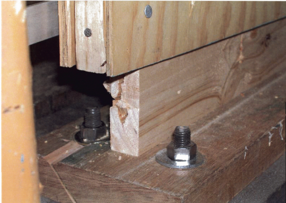
Figure 5.14 Separation on the nail end grain connection for the vertical bottom plate.
