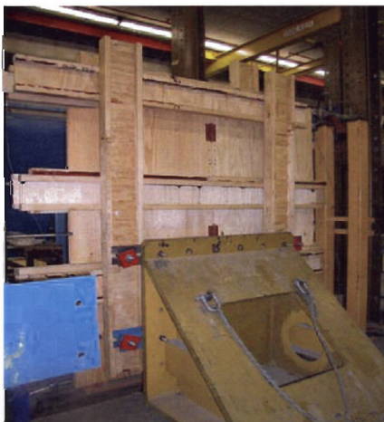
Figure 4.19 Plywood sheathed wall set up for lateral resistance test (see Figure 4.20 for details).
