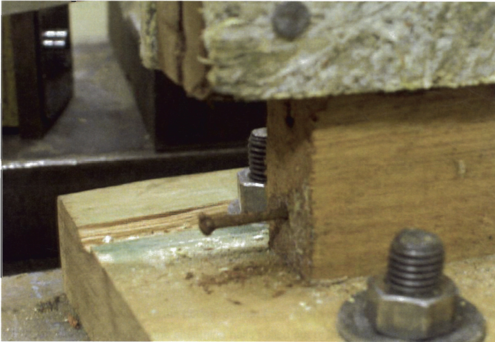
Figure 5.10 Separation of the vertical frame from the base of the wall.
