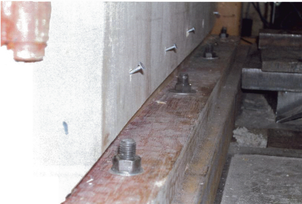
Figure 5.12 Nail pull-out from the timber framing.
