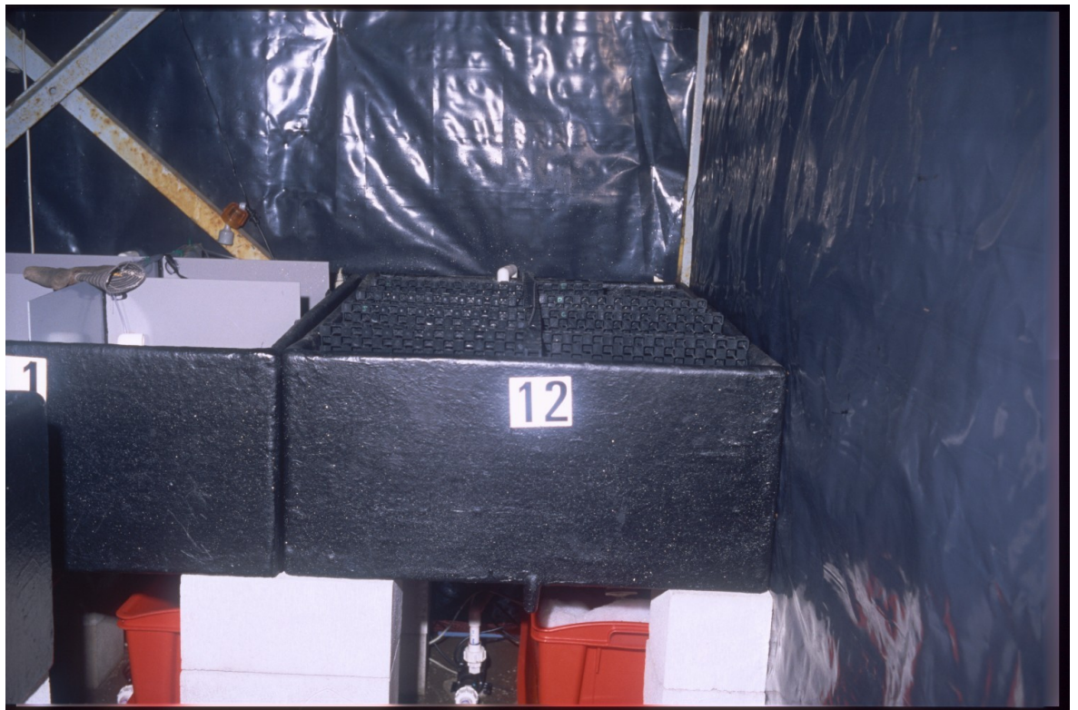
Plate 10. Holding tanks. * Note individual holding tank on the left and flow through cells on the right. The filter, reservoir and pump can be seen under the tank.
