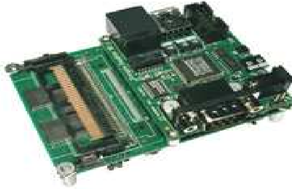
Figure 5.4 Stargate: X-Scale Single Board Computer and Wireless Networking Platform (Crossbow Technology Inc., 2005)
