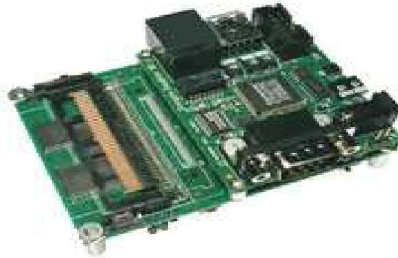
Figure 7.4 Stargate: X-Scale Single Board Computer and Wireless Networking Platform (Crossbow Technology Inc., 2005)
