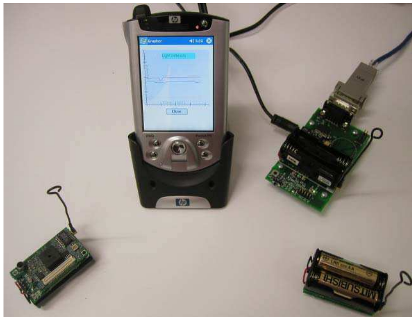
Figure 7.7 Stargate MoteCare Showing Graphs (note the cable from the Stargate is plugged into the PDA charger in this photo)
