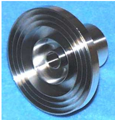
Figure 3.19: 20 GHz compact multi-mode horn antenna for FedSat (Photo: CSIRO)
