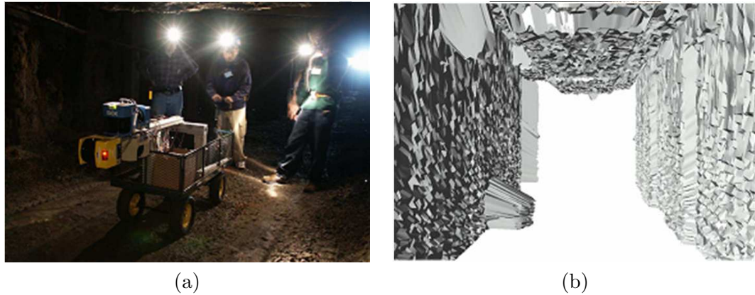
FIGURE 2.1: 3D mapping with a mobile robot [1]. a) Mine mapping cart with four laser range finders; b) Volumetric surface map visualisation using scan matching techniques.
