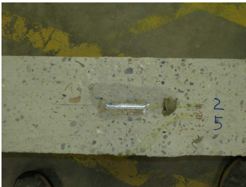
Figure 3.6 A strain gauge for recording strain of concrete
