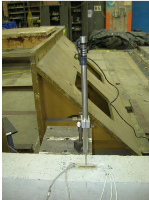
Figure 3.7 A displacement transducer (LVDT) used for displacement monitoring
