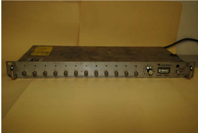
Figure 7.7 Multi-channel signal conditioner
