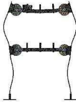
Figure 5.30 New mode (mode 2a) of numerical two-storey framed structure that emerges when mass is added to the upper crossbeam.
