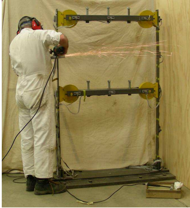
Figure 4.26 Cutting of damage using a disk grinder.
