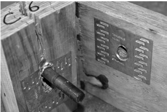
Figure 6 – reinforced LVL connection
