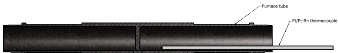
Figure 3.1. Cross sectional view of the temperature measurement setup of the graphite furnace tube using Pt/Pt-Rh thermocouple encased inside an alumina tube.
