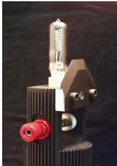
Figure 1.5. FEL lamp used as irradiance spectral standard.
