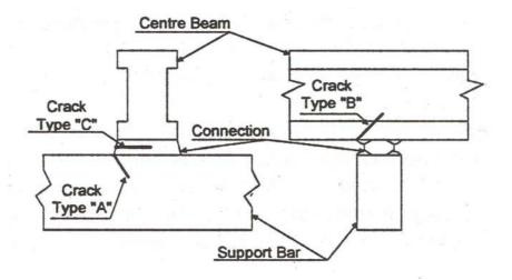
**Figure 3.3** Established fatigue crack patterns – multiple support bar designs
