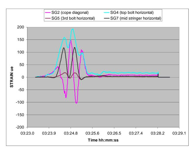
Figure 35 Typical Strain Time Histories – Pre Modification (Ambient Traffic)
