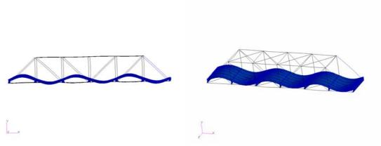
Figure 9 Mode 6 at 13.3 Hz
