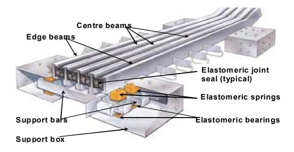
**Figure 1.2** Example of a multiple support bar MBEJ design
