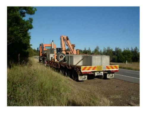
Figure 21 Bridge Load Test Truck
