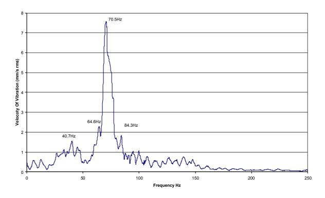
Figure 3: Centre Beam Vibration Spectrum – Anzac Bridge
