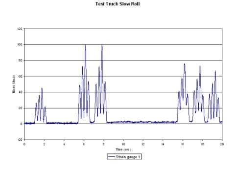
Figure 3.8 Quasi-static strain
