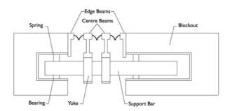
Figure 1 Typical Single Support Bar Design MBEJ
