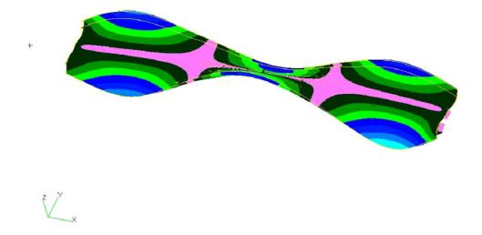
Figure 22 Mode 4 at 6.7 Hz
