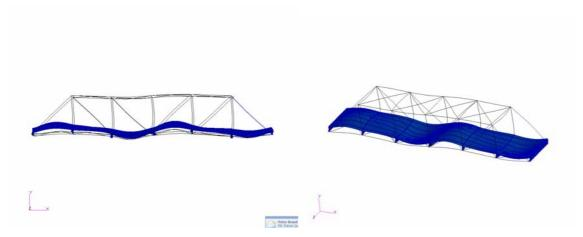
Figure 7 Mode 4 at 10.1 Hz
