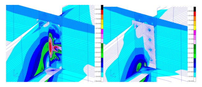
Figure 34 Sample Stress Contour Plots: 2 rows bolts removed left: 4 rows bolts removed right
