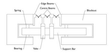
Figure 1 Typical Single Support Bar Design MBEJ
