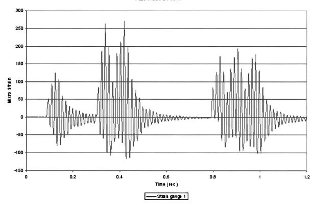
Fig. 12. Response induced by heavy vehicle pass-by
