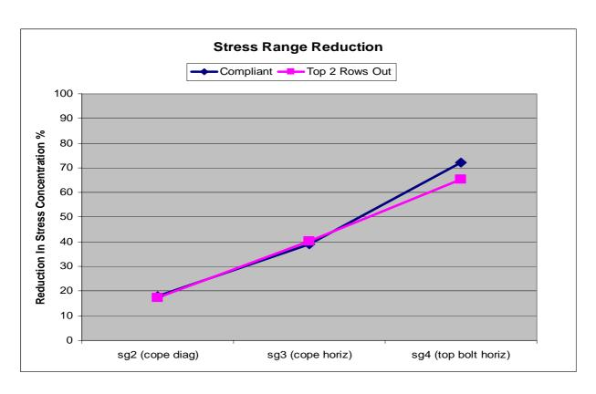
Figure 37 Typical Stress Range Reduction
