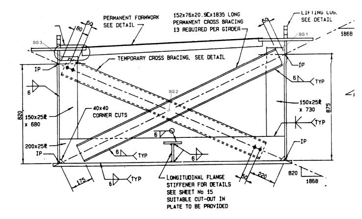
Figure 2 Asymmetric Internal Stiffeners
