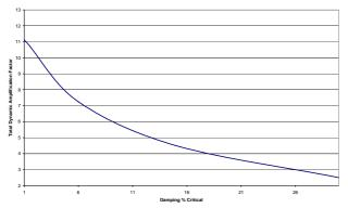
Figure 8 Dynamic Amplification Factor vs Damping (Anzac)
