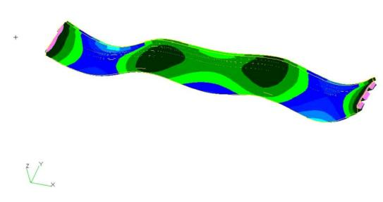
Figure 21 Mode 3 at 5.2 Hz
