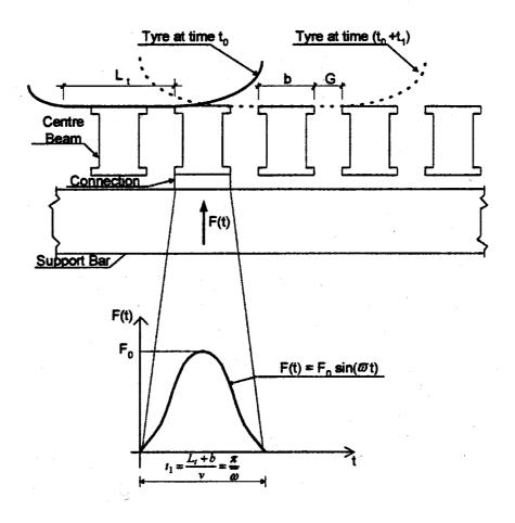
**Figure 4.1** Characteristic half-sine wave impulsive load
