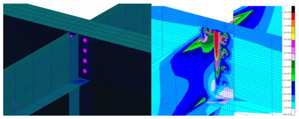
Figure 31 Fine Mesh Model For As Built Connection Detail, base model left, Stress contour results right.
