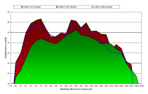
Figure 6: RMS Average Third Octave Band Noise Spectra at Location 4
