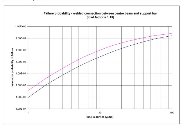
Figure 10 Time-dependent failure probability for a welded connection between center beam and support bar – OEM Condition
