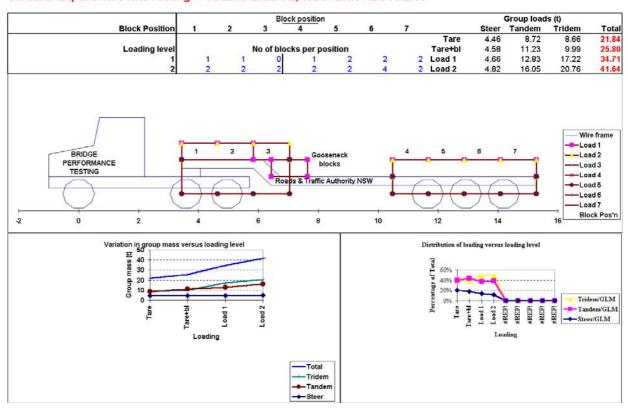
Figure 5 Test Vehicle Loading Arrangement
