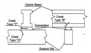
Figure 2 Established Fatigue Crack Patterns – Multiple Support Bar Designs (After Dexter *et al*)
