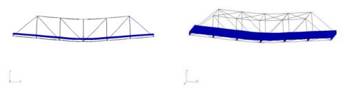
Figure 4 Mode 1 at 3.8 Hz
