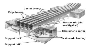
Fig. 1. Example of a multiple-support bar MBEJ system
