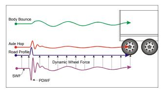
Figure 5 Axle-hop, body-bounce movements and tyre forces induced by a 1.5 m long 40 mm high hump – quarter truck simulation at 80 km/h (After [17])
