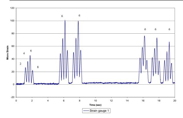
Figure 8 Quasi-static response due to test vehicle pass-by (Contacted center beams shown numbered)
