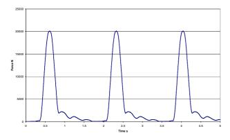
Figure 6 Plot of Virtual Wheel Load Force Profile
