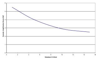
Figure 9 Dynamic Amplification Factor vs Damping (Taree)
