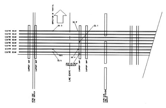
Fig. 8. Plan view eastbound curbside lane—six strain gage locations (SG1 to SG6)
