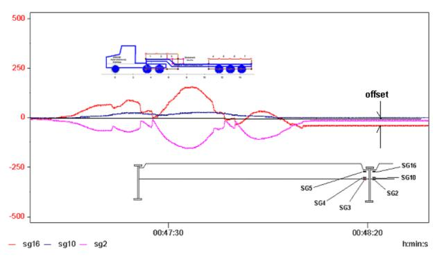
Figure 28 Slow Roll Strain time Histories For Group 4 Gauges, (stringer line 3)
