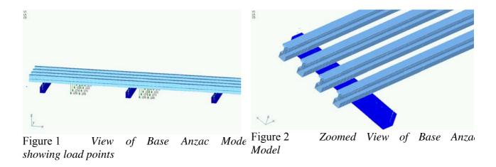
**Figures 1 and 2** show a perspective view including wheel load points and a zoomed view of the base model. It is important to note that the emphasis of dynamic analysis was on the vertical response of the structure (i.e. any resulting horizontal centre beam bending modes have not been reported). Based on the results of investigations to date, horizontal modes were not found to be particularly relevant to the major dynamic loads developed during traffic excitation.
