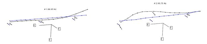
Figure 14 - - Mode shapes of one centerbeam & support bars for truck tire excitation.
