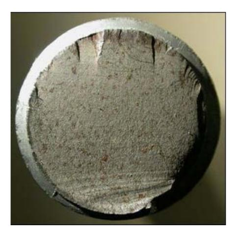
Figure 2 Fatigue affected bolt
