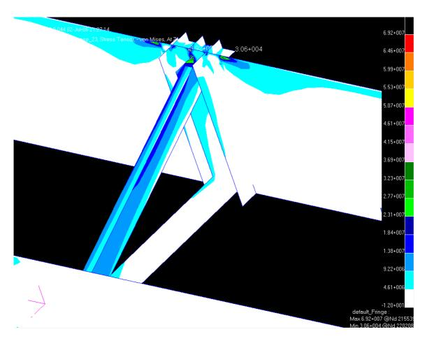
Figure 24 Sample Stress contour Plot, Three Rib Bolted Stiffener
