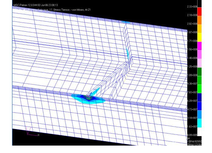
Figure 23 Sample Stress Contour Plot Of Box Girder, As Built Condition
