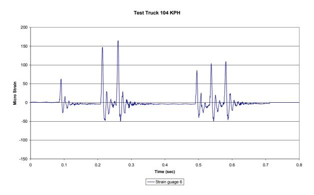
Figure 8 - Time domain response of a support bar at 104 km/hr (Taree)
