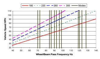
Figure 6 Calculated Beam Pass Frequencies for a Range of Expansion Joint Spacings
