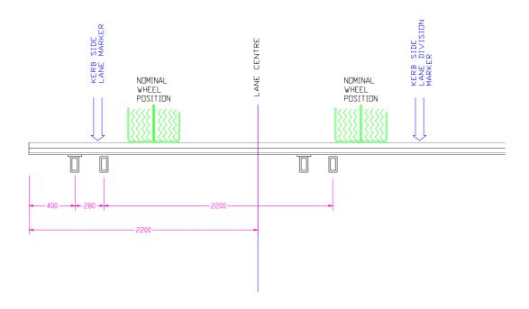
**Figure 3.11** Elevation of modular expansion joint and nominal test truck position
