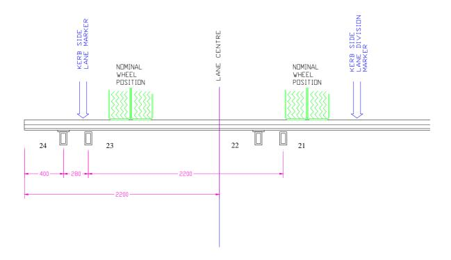
Figure 6 Elevation of Joint and Nominal Pass-by Locations (Support bars shown numbered)
