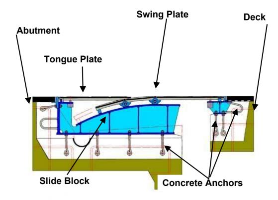
Figure 1.1 Typical cross-section of a roller shutter joint
