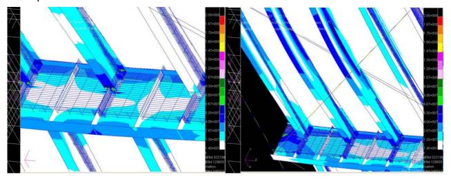
Figure 32 Sample Stress Contour Plots For Stringer top Plate replacement Option
