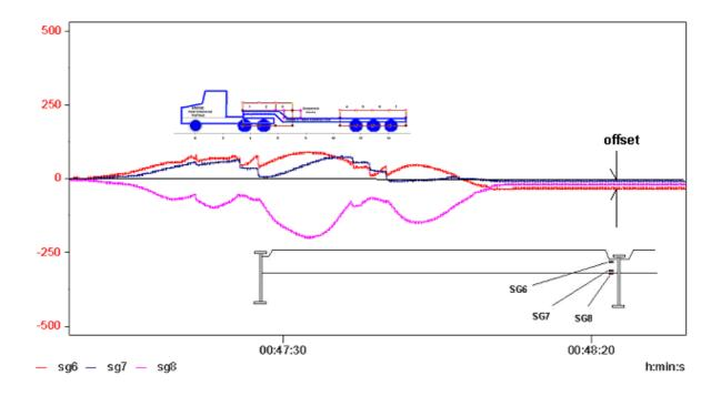
Figure 29 Slow Roll Strain time Histories for Group 5 Gauges, (stringer line 2, see also Figure 19 for locations)
