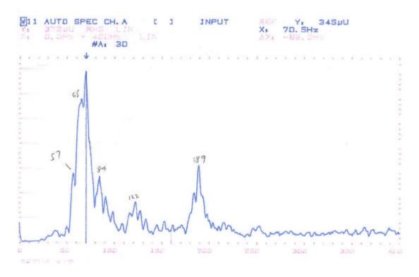
Figure 5: Transverse Beam Vibration Spectrum – Anzac Bridge
