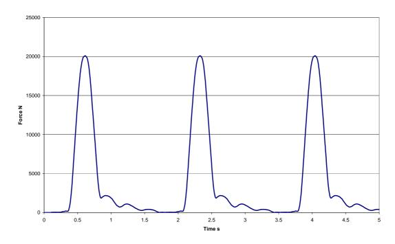
Figure 3.5 Plot of virtual wheel load force profile
