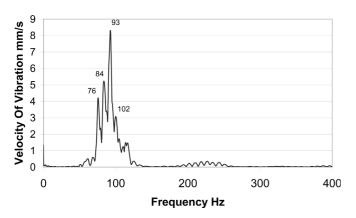
Figure 3 Centre Beam Vibration Spectrum - Tom Ugly's Bridge
