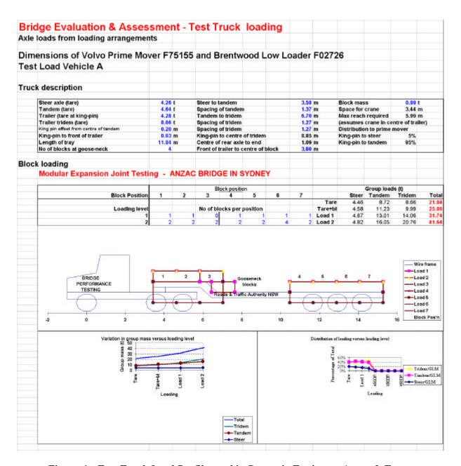
Figure 6: Test Truck Load Profile used in Dynamic Testing at Anzac & Taree
