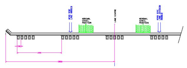
Figure 6 - Truck position on joint, Taree Bypass - Strain Gage Testing
