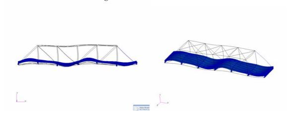
Figure 7 Mode 4 at 10.1 Hz
