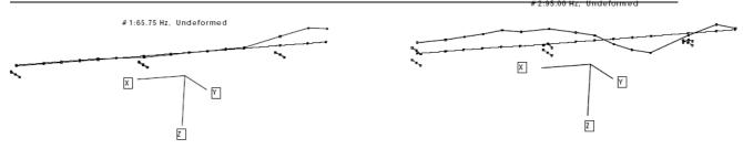
Figure 13 - Mode shapes of one centerbeam & support bars for hammer pulse excitation.
