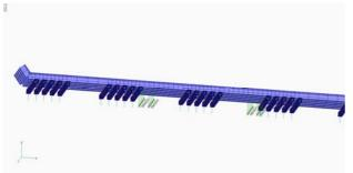
Figure 3 View of Base Taree Model showing load points
