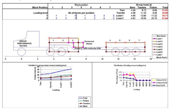
Figure 20 Test Vehicle Loading Arrangement
