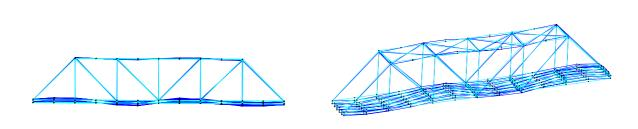
Figure 16 Mode 4 at 10.16 Hz Fourth Vertical Bending, (5 nodes)
