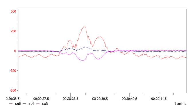
Figure 30(b) Sample Strain Time History Module 5 Gauges, 59km/hr
