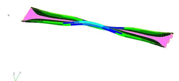
Figure 20 Mode 2 at 4.8 Hz
