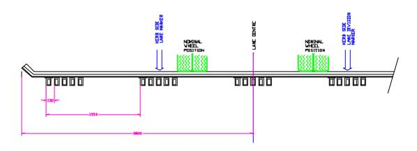
Figure 8: Elevation of MBEJ and Nominal Test Truck Position (Taree)
