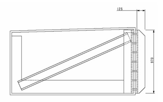
Figure 26 Drawing of Single Rib Welded Stiffener
