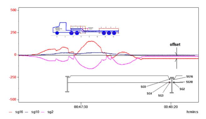
Figure 28 Slow Roll Strain time Histories For Group 4 Gauges, (stringer line 3, see also Figure 19 for locations )
