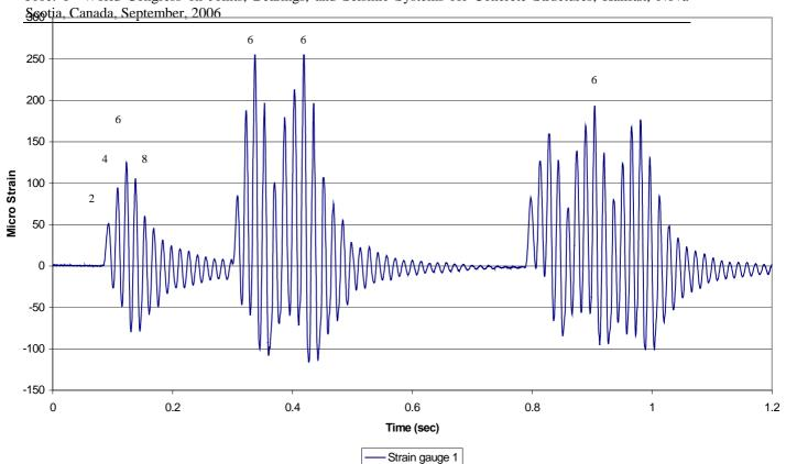
Figure 9 Dynamic response induced by heavy vehicle pass-by at 61 km/hr (Contacted center beams shown numbered)
