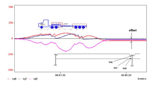
Figure 29 Slow Roll Strain time Histories for Group 5 Gauges, (stringer line 2)
