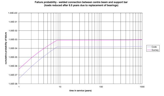
Figure 11 Time-dependent failure probability for a welded connection between center beam and a support bar – Prototype #3
