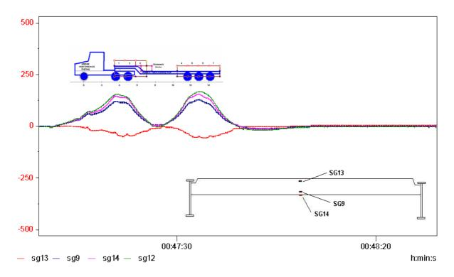
Figure 26 Slow Roll Strain time Histories For Group 2 Gauges, (SG9, SG13 and SG14 on stringer line 3, SG12 as SG14 but on stringer line 2, see also Figure 19 for locations)
