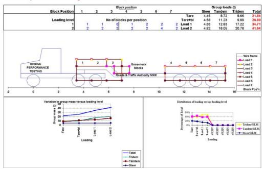
Figure 3.10 Test vehicle loading arrangement
