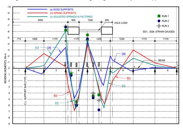
Figure 5 – Bending Moment Diagrams based on Static Analysis
