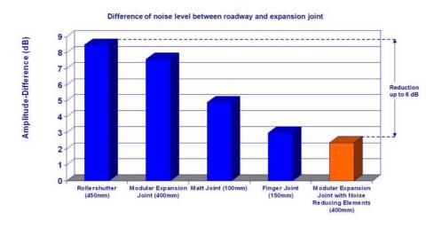
**Figure 2.4** Noise reduction comparison (Courtesy Mageba SA)
