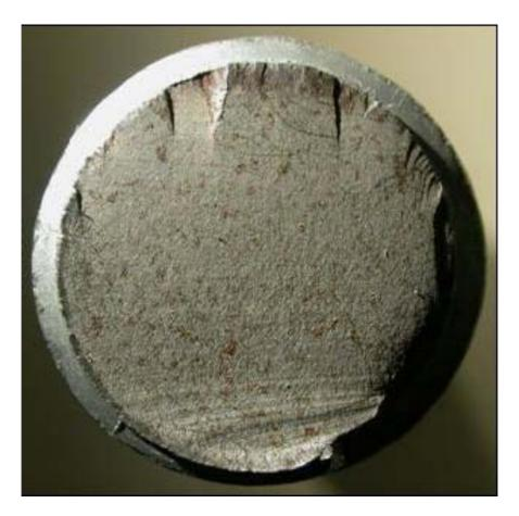
Figure 2 Fatigue affected bolt
