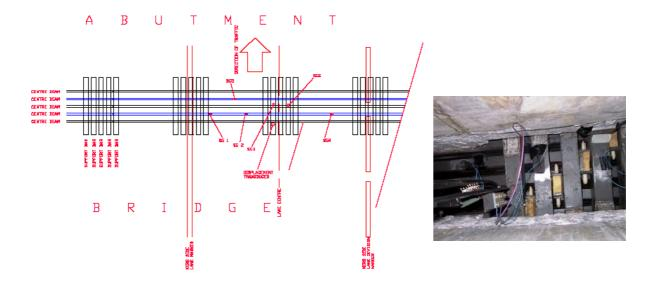
Figures 4 and 5 - Strain gage layout on the Taree Bypass structure
