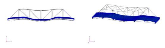
Figure 6 Mode 3 at 9 Hz
