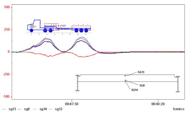
Figure 26 Slow Roll Strain time Histories For Group 2 Gauges, (SG9, SG13 and SG14 on stringer line 3, SG12 as SG14 but on stringer line 2)
