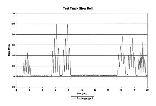
Fig. 13. Quasi-static response due to test vehicle pass-by
