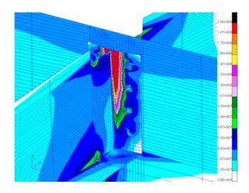
Figure 33 Sample Stress Contour Plot, Compliant Connection Option
