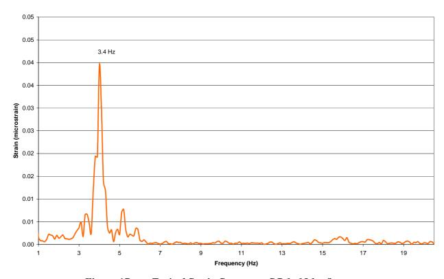
Figure 17 Typical Strain Spectrum; SG 1; 15 km/hr
