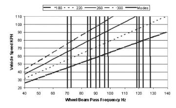
**Fig. 7.** Calculated wheel beam pass frequency for a range of expansion joint spacings
