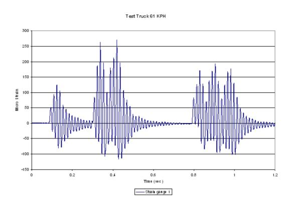
**Figure 3.7** Coupled centre beam resonance
