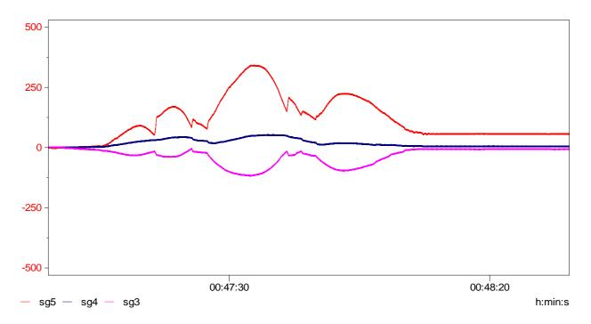
Figure 30(a) Sample Strain Time History Module 5 Gauges, slow roll
