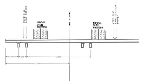
Fig. 10. Elevation of modular expansion joint and nominal test truck position
