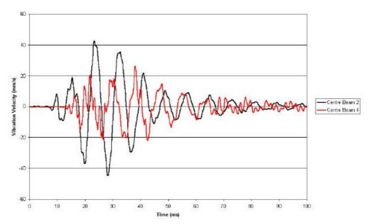
Figure 16 - Time domain plot characterizing centerbeam cross coupling
