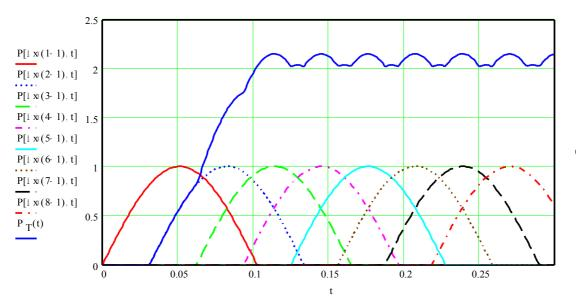
Figure 12 – Pulse train for FEA modeling. Note the pulses should add to 1.0 when the joint is fully loaded, hence the need for the pulse scale factor, A.
