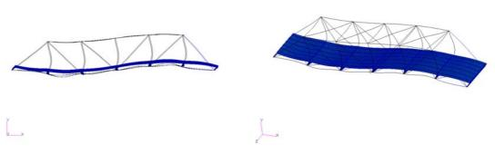
Figure 5 Mode 2 at 7 Hz
