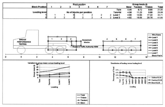
Fig. 9. Test vehicle loading arrangement
