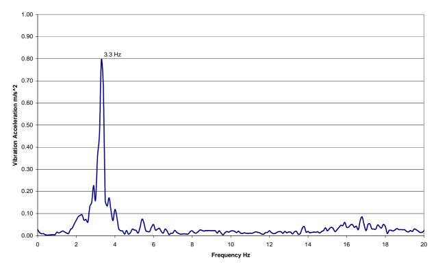
Figure 18 Test Truck Vertical Chassis Vibration Spectrum (Bump Test)
