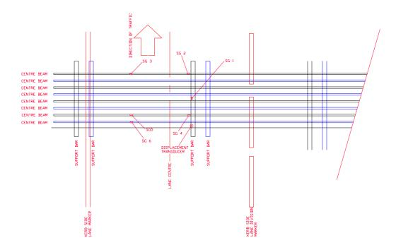
**Figure 3.9** Plan view eastbound kerbside lane - six strain gauge locations (SG1 to SG6)
