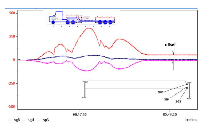
Figure 27 Slow Roll Strain time Histories For Group 3 Gauges, (stringer line 3, see also Figure 19 for locations)
