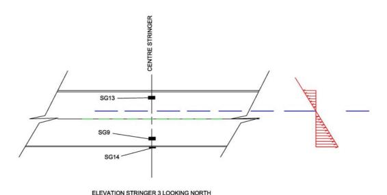
Figure 24 Stringer Diagrams Showing Measured Position of Neutral Axis
