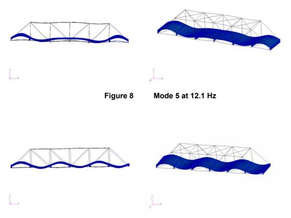
Figure 9 Mode 6 at 13.3 Hz
