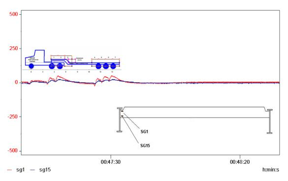
Figure 25 Slow Roll Strain time Histories For Group 1 Gauges, (stringer line 3, see also Figure 19 for locations)
