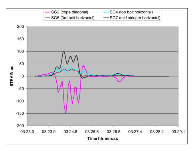
Figure 36 Typical Strain Time Histories – Post Modification (Ambient Traffic)
