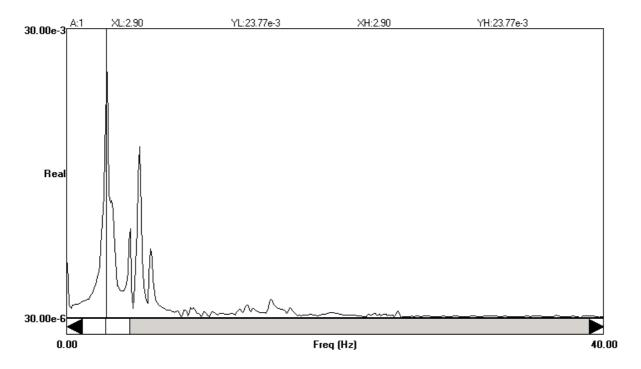
Figure 8 Typical Narrow Band Vibration Spectrum (Cursor at 2.9 Hz)
