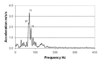
Fig. 4. Center beam vibration spectrum, Anzac Bridge
