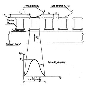
Figure 7 Characteristic Half-Sine Wave Impulsive Load
