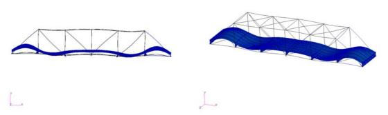
Figure 8 Mode 5 at 12.1 Hz
