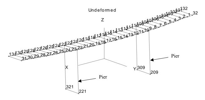
Figure 7 Line Drawing of the Undeformed Structure showing Measurement Locations
