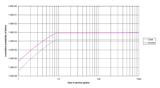
Figure 3.14 Time-dependent failure probability for a welded connection between centre beam and a support bar – prototype #3
