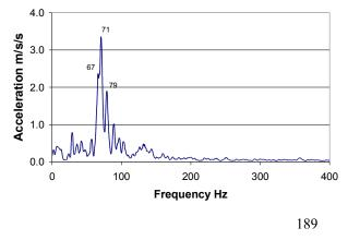
Figure 8 Centre Beam Vibration Spectrum – Anzac Bridge
