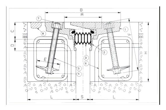
Figure 2.5 Sealed aluminium finger joint [after Watson & Delattre (2008)]
