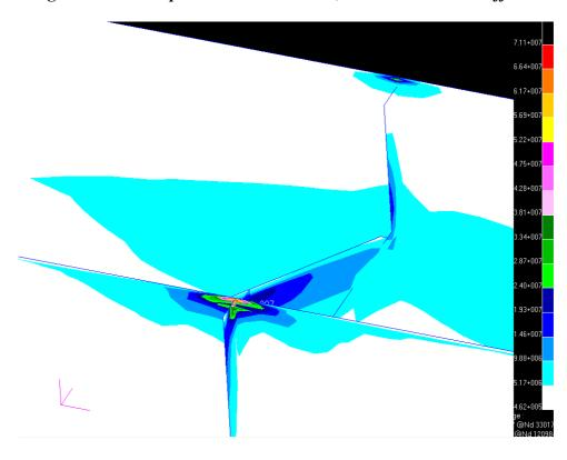
Figure 25 Sample Stress Contour Plot, Single Rib Welded Stiffener
