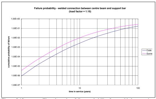
Figure 3.13 Time-dependent failure probability for a welded connection between centre beam and support bar – OEM condition
