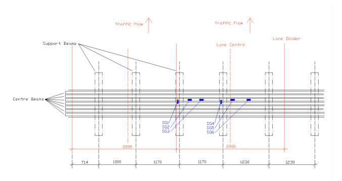
Figure 4 Plan View Southbound Curbside Lane - Six Strain Gage Locations (SG1 to SG6)
