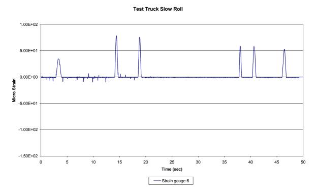
Figure 7 - Time domain response of a support bar at slow roll (Taree)
