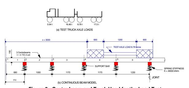
Figure 2 - Centre beam and Truck Used for the Load Test
