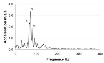
Figure 5 Centre Beam Vibration Spectrum - Anzac Bridge
