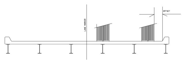
Figure 22 Sectional Elevation of Bridge Deck Showing Nominal Test Truck Position
