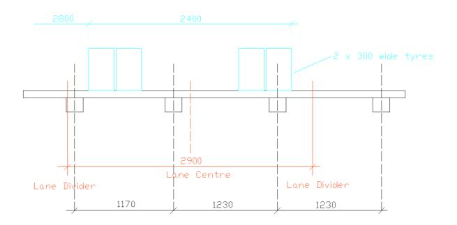
Figure 5 Elevation of Modular Expansion Joint and Nominal Test Truck Position
