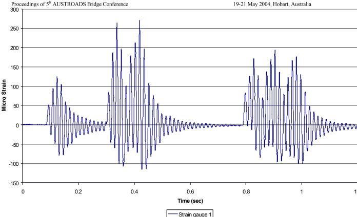
Figure 10: Dynamic response induced by heavy vehicle pass-by (Anzac)
