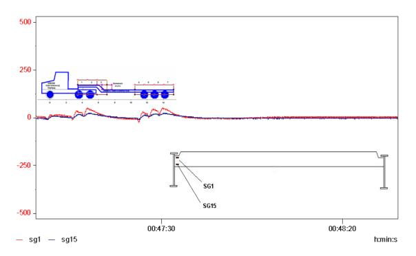
Figure 25 Slow Roll Strain time Histories For Group 1 Gauges, (stringer line 3, see also Figure 19 for locations)
