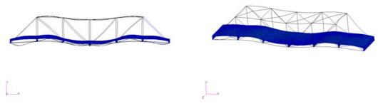
Figure 6 Mode 3 at 9 Hz
