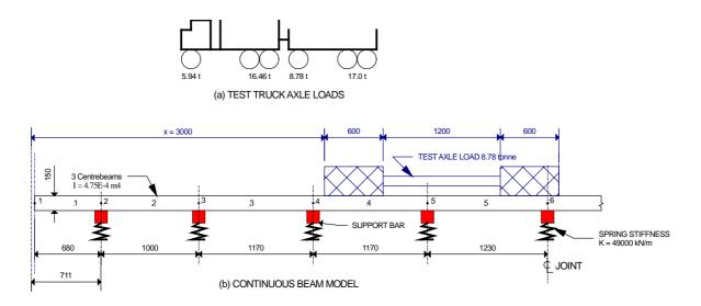
Figure 3 Center beam and Truck Used for the Load Test
