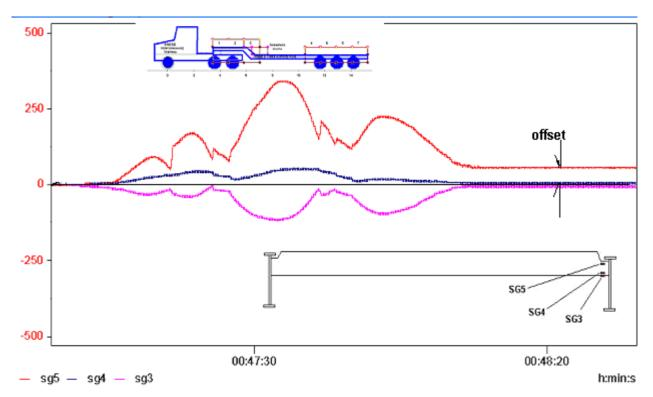
Figure 27 Slow Roll Strain time Histories For Group 3 Gauges, (stringer line 3)
