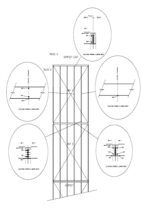
Figure 19 Plan View North Bound kerbside Lane - Sixteen Strain Gauge Locations (SG1 to SG16)
