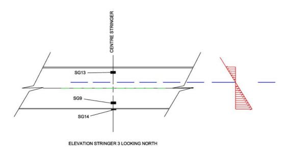
Figure 24 Stringer Diagrams Showing Measured Position of Neutral Axis
