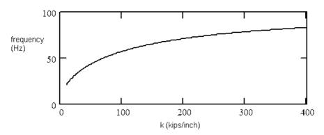
Figure 15 - Plot showing the vertical fundamental joint frequency versus bearing stiffness (Eq. 19)
