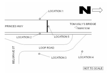
Figure 6 Site Plan Showing Noise Measurement Locations
