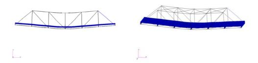
Figure 4 Mode 1 at 3.8 Hz
