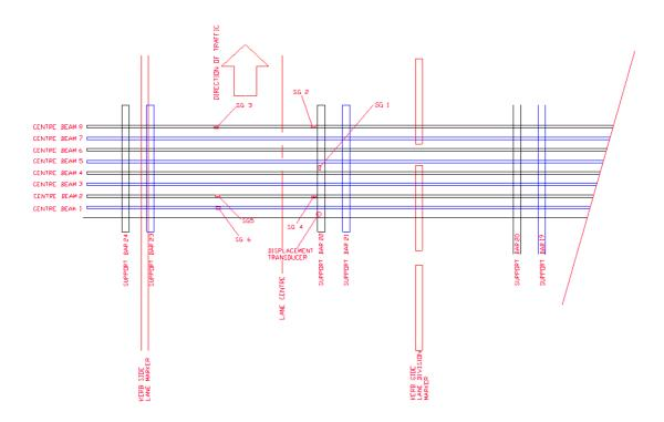
Figure 4 Eastbound Carriageway - Strain Gage Locations (SG1 to SG6)
