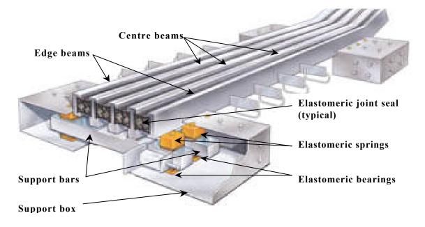
Figure 2: Typical Multiple Support Bar Design MBEJ
