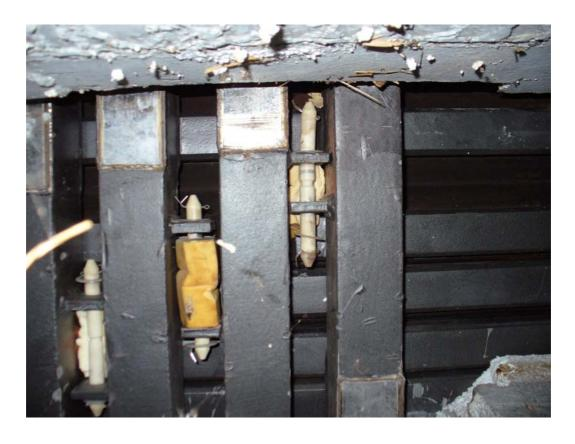
**Figure 1.5** Failed elastomeric springs at Taree (NSW) also showing compression set
