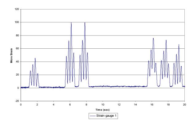
Figure 9 – Static response induced by heavy vehicle slow roll (Anzac)
