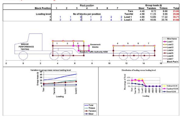
Figure 20 Test Vehicle Loading Arrangement
