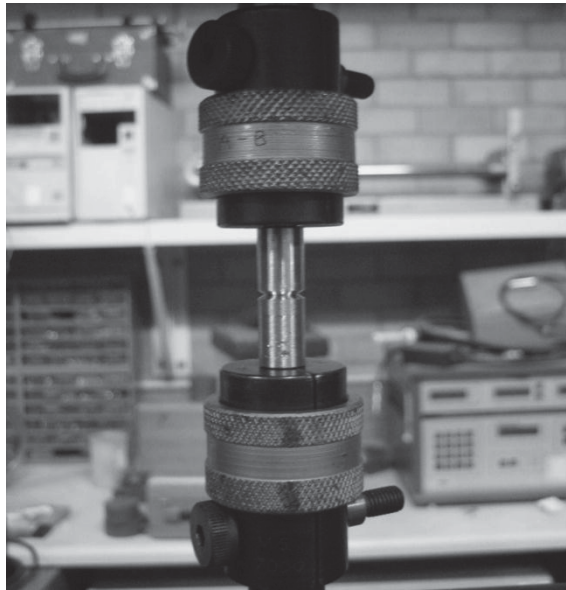
Figure 6–10. Circumferential notch tension test (a) specimen held by split-collet grips.
