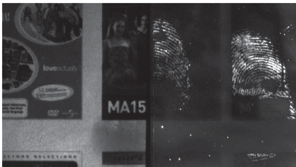
Figure 4.11. left: Fresh fingerprints (<2 hrs old) developed on glossy magazine paper. (left) CAF and rhodamine 6G staining, illuminated at 530 nm and with a 610 nm band pass filter; (right) \text{YVO}_4:\text{Er,Yb} dry-powdered, illuminated using a 980 nm laser pointer with a 555nm band pass filter.
