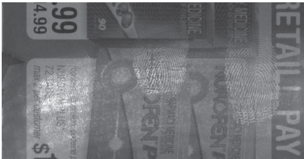
Figure 3.7. Fresh fingermark on magazine paper developed by dry powdering method of UC particles, under the illumination of 980 nm laser pointer with a 555nm band pass filter and 10.3 s exposure time.
