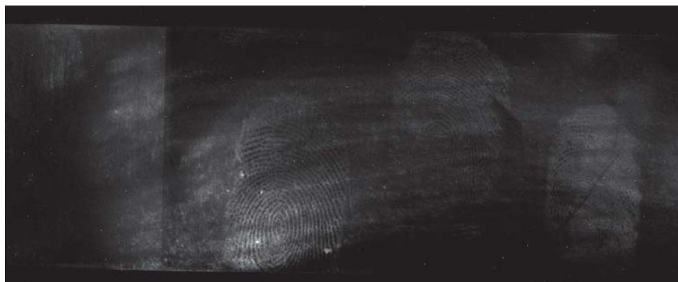
Figure 6.8. Fresh fingerprints developed by UC-PEI particles on a glass slide (applied as a dry powder). Illuminated with a 980 nm laser light and imaged using a Rofin Poliview fitted with a 555nm band pass filter and using an exposure time of approximately 10 seconds.
