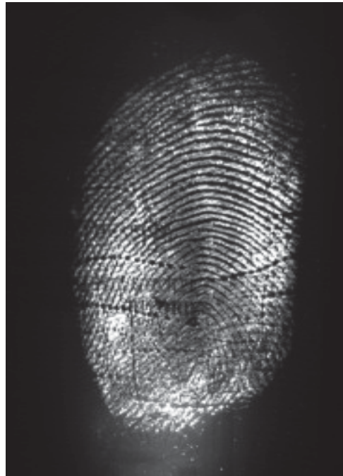
Figure 4.6. Fresh fingerprint (< 2 hrs old) on an Australian five dollar polymer banknote developed with \text{YVO}_4:\text{Er},\text{Yb} dry powdering. Illuminated at 980 nm and imaged with a 555nm band pass filter. The absence of visible background should be noted.
