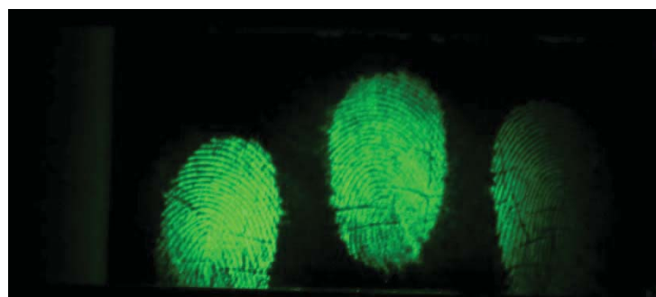
Figure 2.6. Fresh fingerprints on glass developed by \text{NaYF}_4:\text{Er,Yb} dry powdering, under the illumination of The Crime-Lite ASV and imaged using a Canon EOS 450 D SLR camera with F 5.6 and 2.0 second exposure time.
