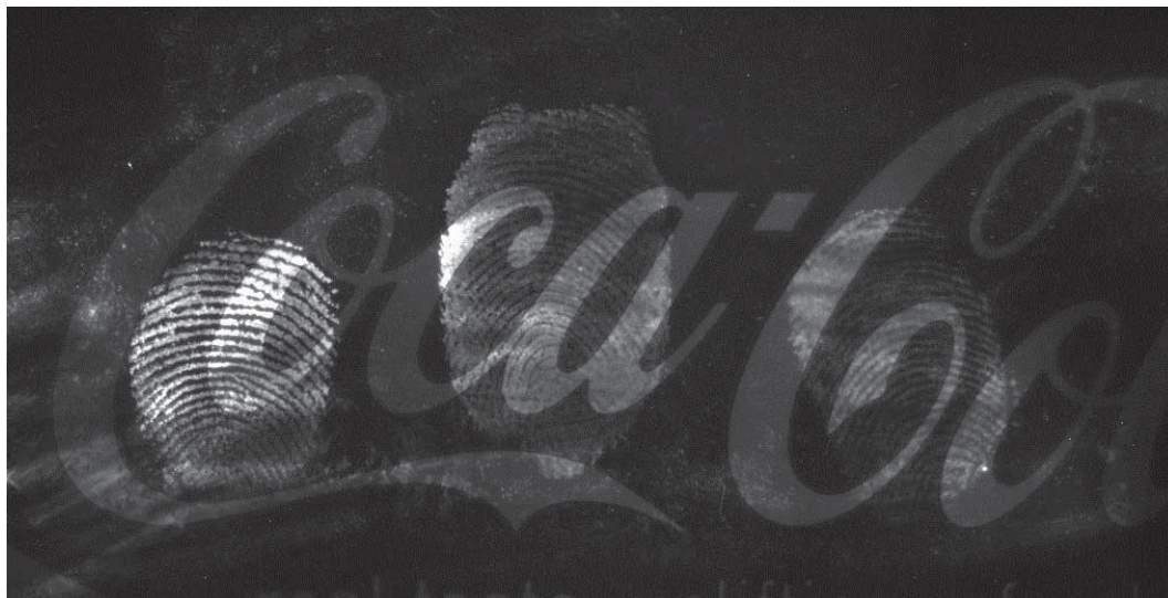
Figure 3.9. Fresh fingerprint on Coca cola plastic tag developed by dry powdering method of UC particles, under the illumination of 980 nm laser pointer with a 555nm band pass filter and 10.3 s exposure time.
