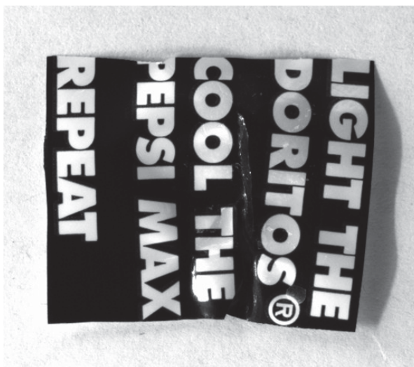
Figure 2.7. A plastic specimen that was deformed by the heat produced by the Crime-Lite ASV.
