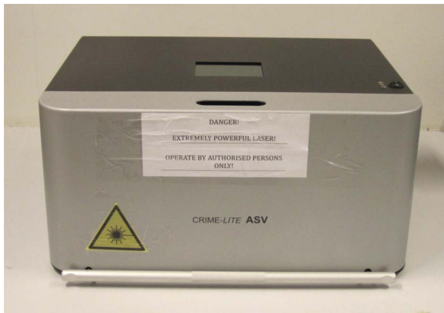
Figure 2.5. The Crime-Lite ASV (Foster and Freeman, UK).
