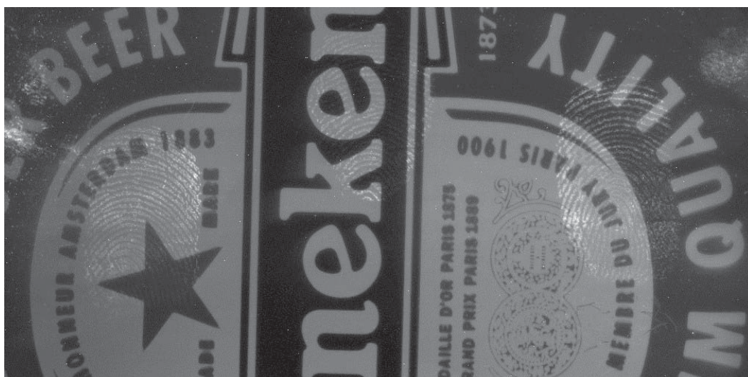
Figure 3.8. Fresh fingermark on beer can developed by dry powdering method of UC particles, under the illumination of 980 nm laser pointer with a 555nm band pass filter and 15.2 s exposure time.
