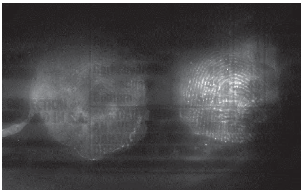
Figure 6.9. Fresh fingerprints on a soft drink can developed with CAF followed by UC-PEI staining. Illuminated using a 980 nm laser pointer with 20s exposure time and imaged using a Rofin Poliview system with a 555nm band pass filter.
