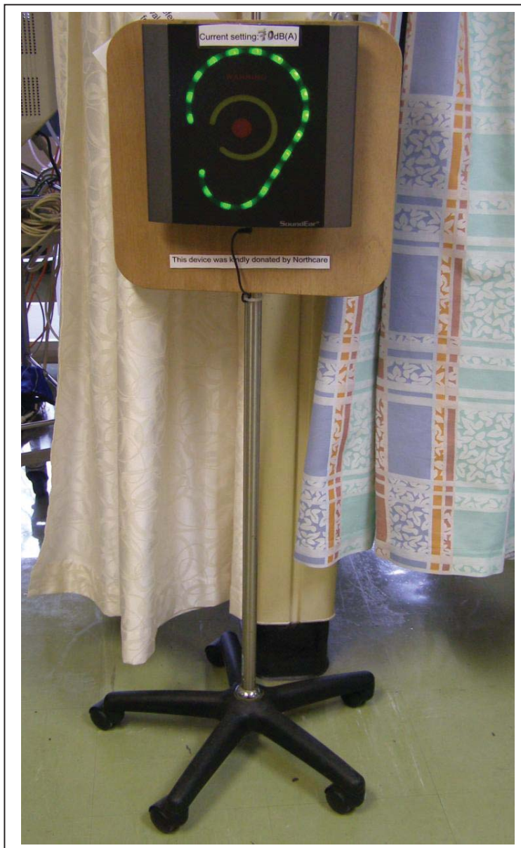
Photograph showing the SoundEar 2000 ® used as a visual reminder of sound pressure levels
