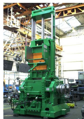
Figure 1.31. Schematic and photograph of Banbury mixer in tire manufacturing. Reproduced from technical document from Farrel corporation.
