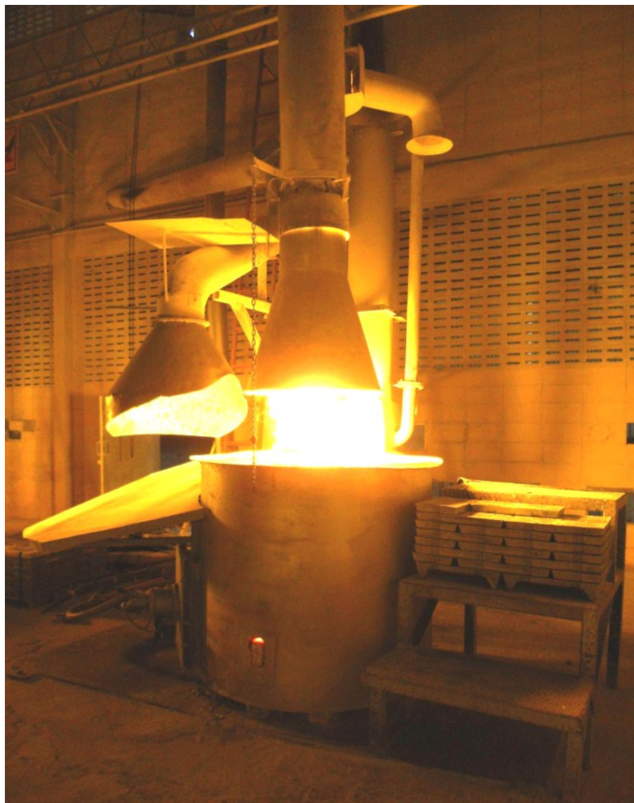
Figure 1.5. Photograph of a French process drum in operation, by permission from PT. Indo Lysaght, Indonesia.
