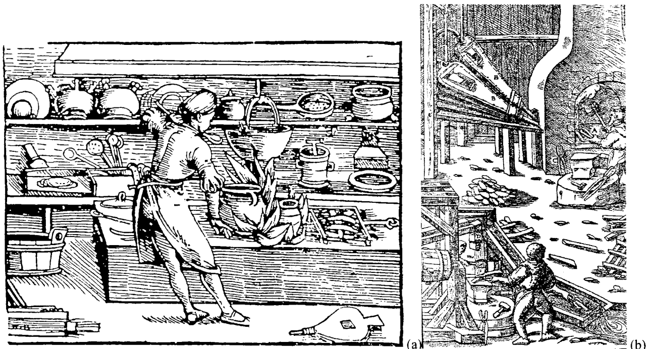
Figure 2. Synthetic jet actuators are the idealization of an old idea, the bellows, which has long been used in both household kitchens (a) 5 and blacksmith workshops (b) 6 .
