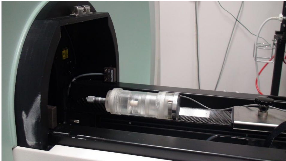
Figure 3.7 Experimental setup showing the placement of the jig in the \mu\text{CT} scanner.
