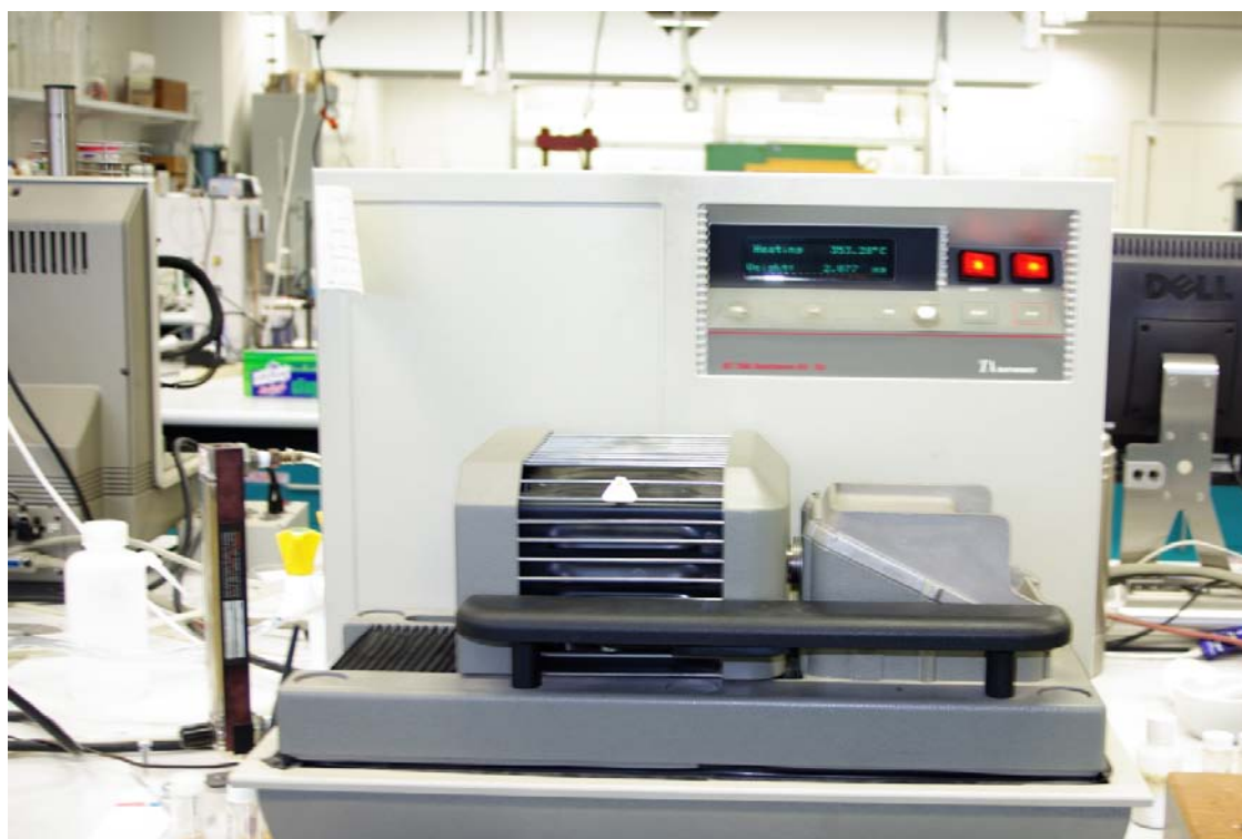
Fig. 3-7 A TGA/DTA Analyzer (SDT 2960 model, TA Instruments). (Image captured from the Science Faculty Resource Manage System, UTS)
