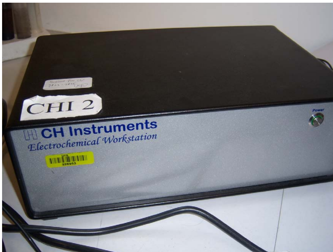
Fig. 3-9 An electrochemistry workstation (CHI660D model).
