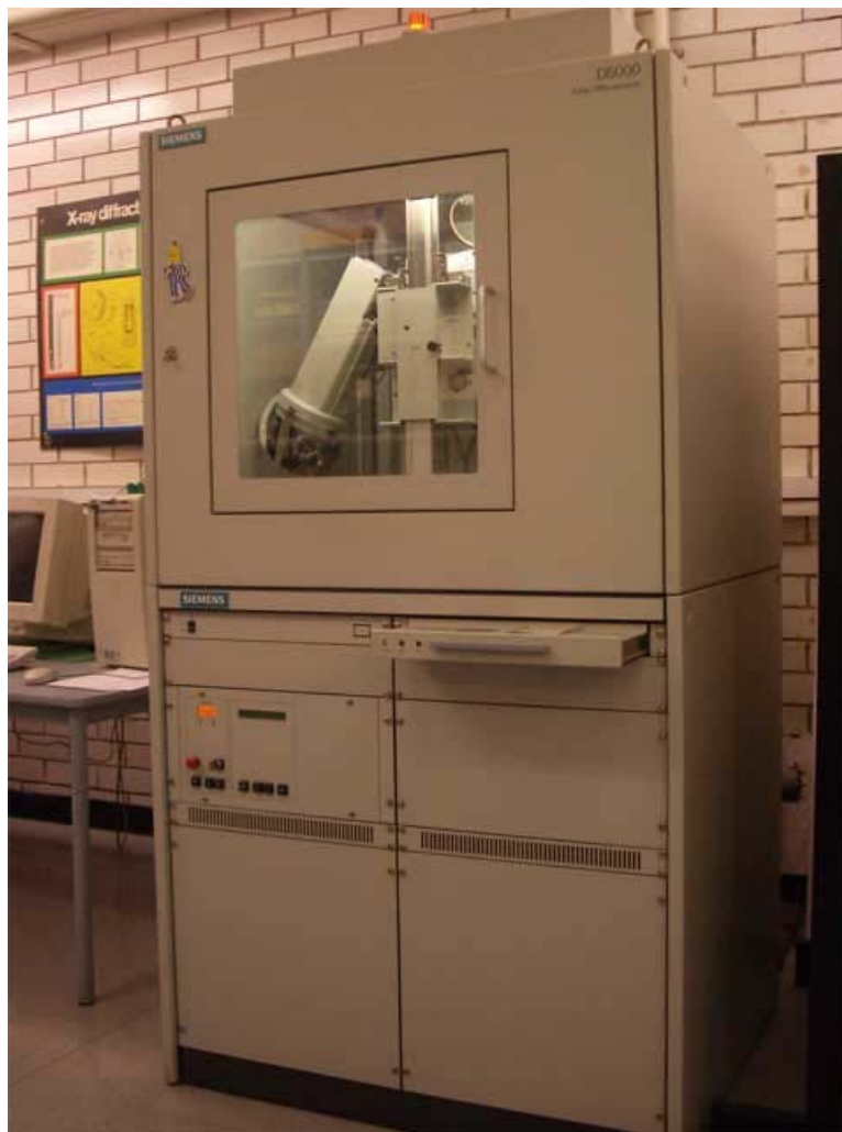
Fig. 3-1 An X-ray diffractometer (Siemens D5000 model). (Image captured from the Science Faculty Resource Manage System, UTS)
