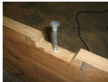
(b) Trapezoidal notch with coach screw
