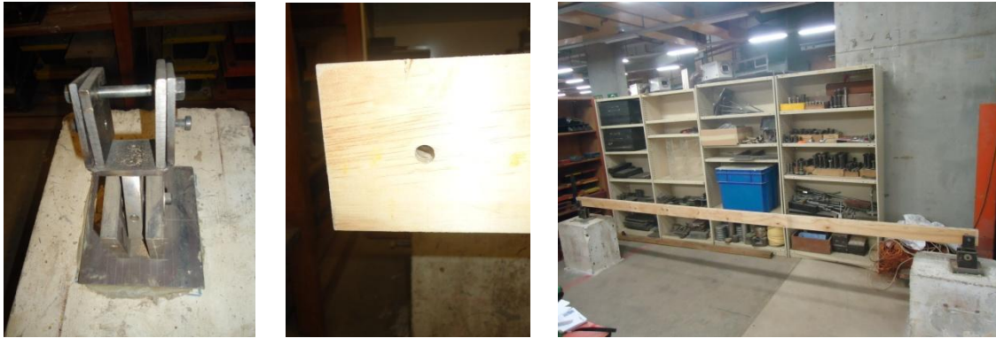
(a) Pin support (b) Hole in web (c) Web element connected to supports
