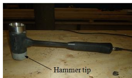
Figure 2.13 A typical impact hammer.
