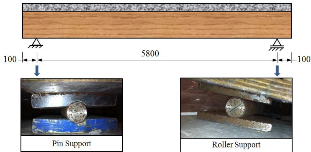
Figure 5.7 Experimental setup for the TCC beams (mm).
