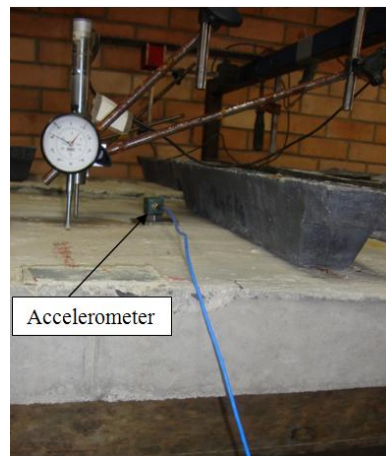
Figure 3.50 Accelerometer model PCB 356A08.
