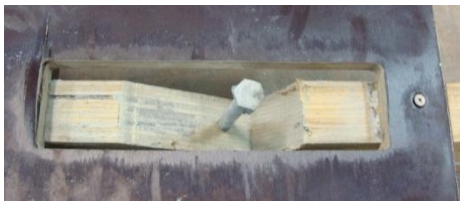
(c) Triangular or bird-mouth notch with coach screw
