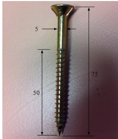
Figure 6.29 Dimensions of the wood screw used to connect the elements of the experimental timber composite beam (mm).
