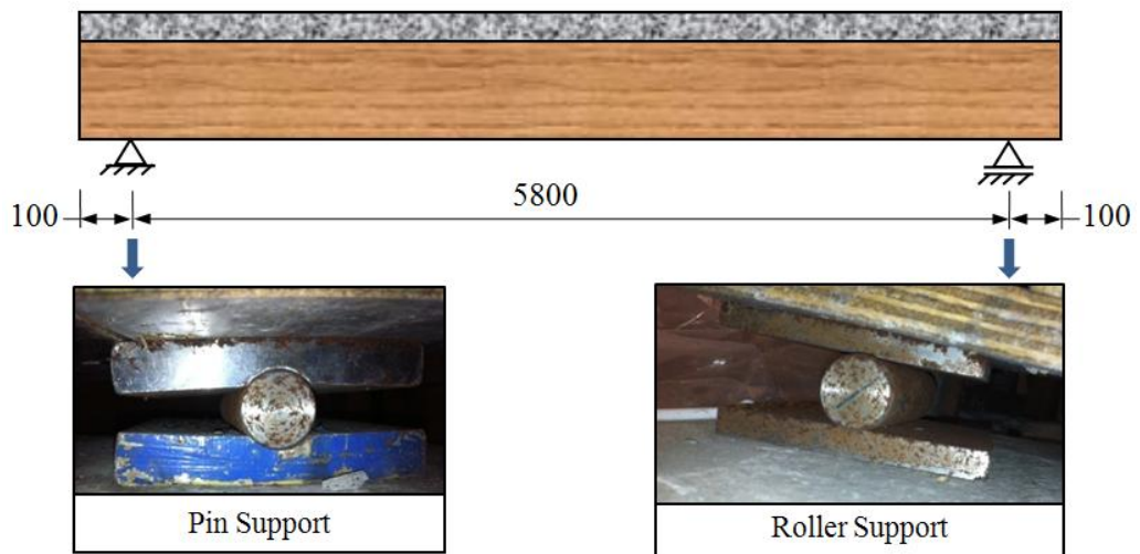
Figure 3.40 Experimental setup for the TCC beams (mm).
