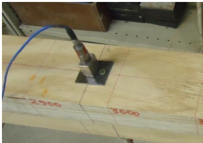
(a) Accelerometer model PCB 352C34
