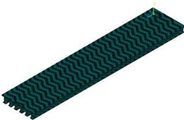
Figure 8.35 A FE model of 8.0 x 1.8 m floor.
