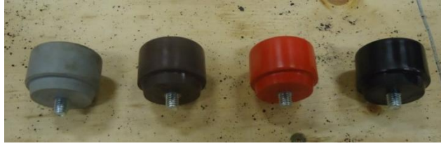
Figure 2.14 Types of hammer tip of a typical hammer.
