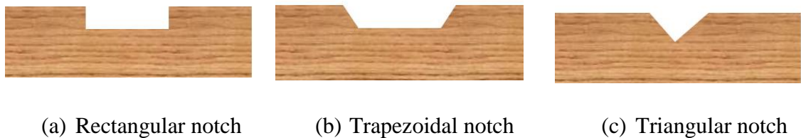
Figure 2.23 Common types of notch connection.
