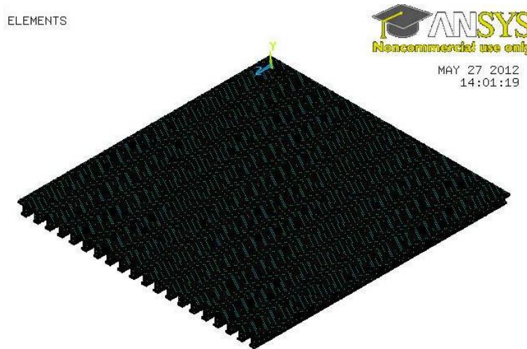
Figure 8.41 A FE model of 6 x 6 m floor.
