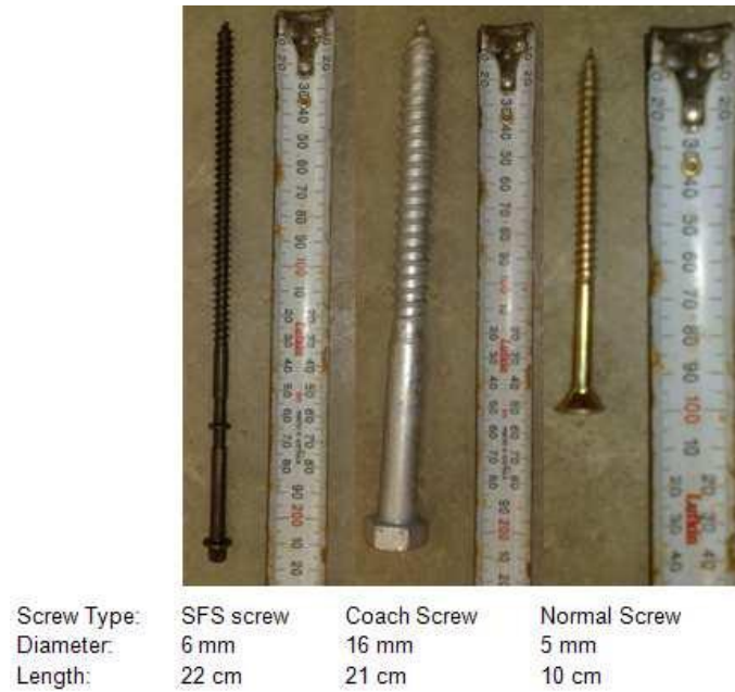
Figure 2.22 Different types of mechanical connectors.
