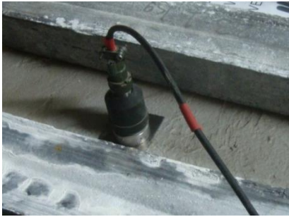
(a) Accelerometer model PCB 337A26
