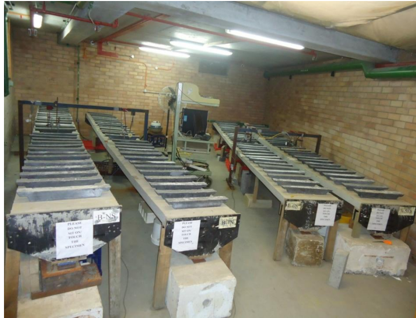
Figure 3.48 Beams under quasi-permanent loads (Hailu et al. 2012).
