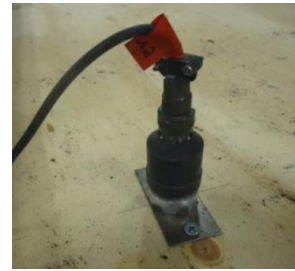
(b) Accelerometer model PCB 337A26
