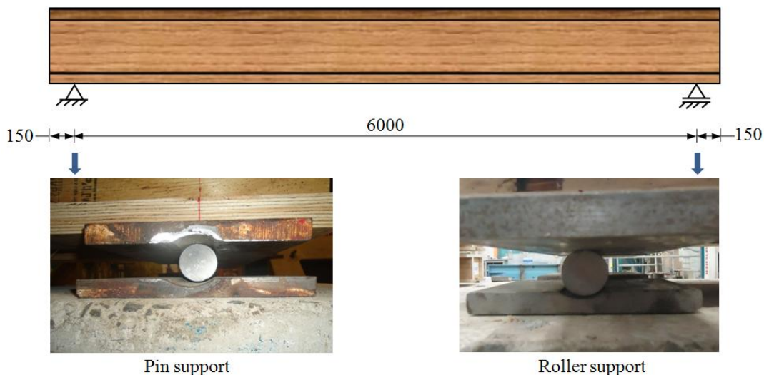
Figure 5.22 Experimental setup for 6 m span beam (mm).
