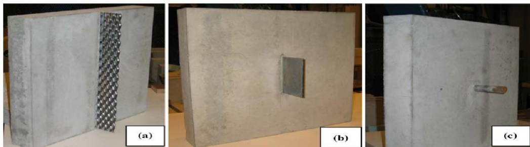
Figure 2.21 Prefabricated concrete slabs with inserted connectors: (a) Continuous steel mesh, (b) Folded steel plate, (c) Steel dowel with flanges (Lukaszewska, Johnsson & Fragiaco 2008).
