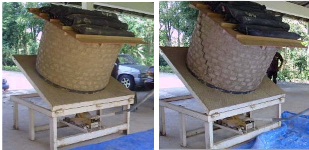
Figure 8.6: Tilting the specimen until cracking and subsequent failure.
