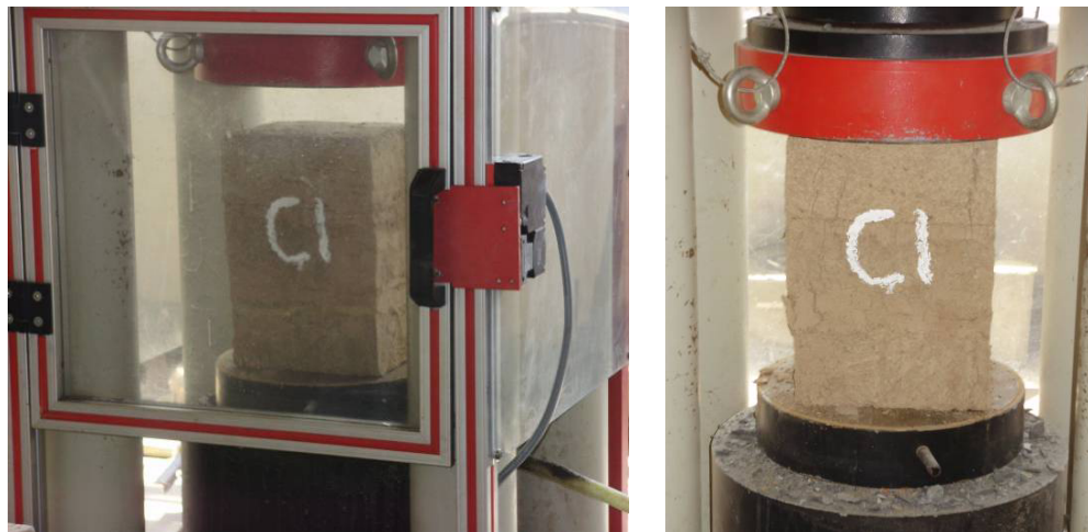
Figure 6.7: Compression test with specimen C1.
