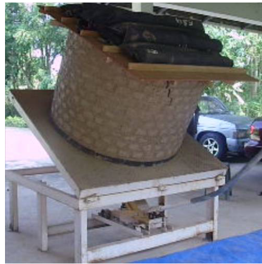
(2) The first cracking appeared.
