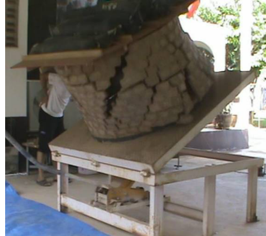
(4) Subsequent total failure.
