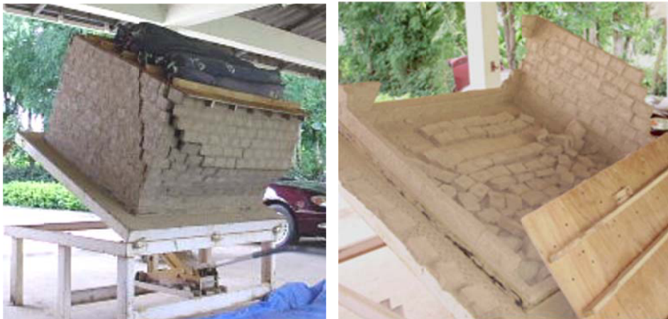
Figure 7.7: The failure modes of the square specimen when tilted further.
