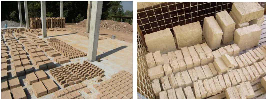
Figure 6.2: Making adobe bricks by mould.
