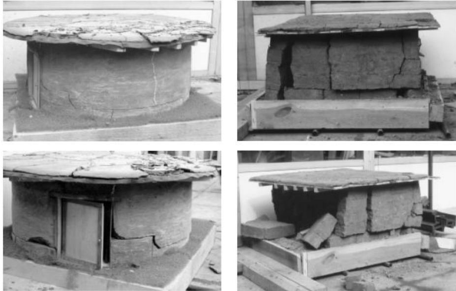
Figure 2.28 : Earthquake resistance of earthen buildings in circular shape (left) and square shape (right)(Minke 2001).
