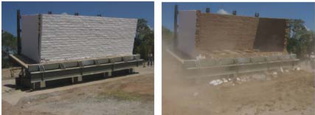
Figure 2.12: The collapses of the front wall of traditional adobe house when tilting reach 14 degrees (Pena & Lopez 2007).
