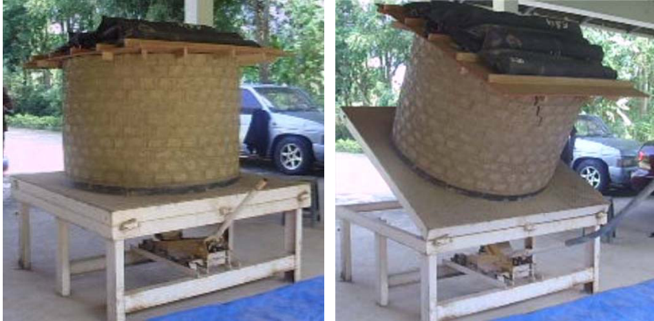
Figure 7.8: Tilting the circular specimen and first crack appearing at 29 degrees.
