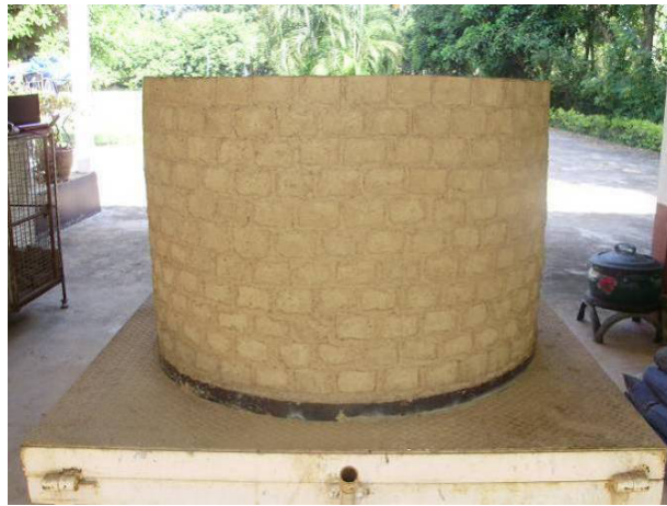
Figure 8.3: Construction of a circular adobe specimen.
