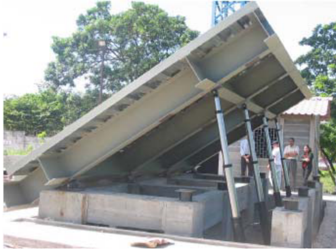
Figure 2.11: Tilt table with 40 degrees as maximum angle(Pena & Lopez 2007).
