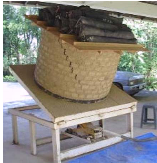
(2)The first crack appeared.
