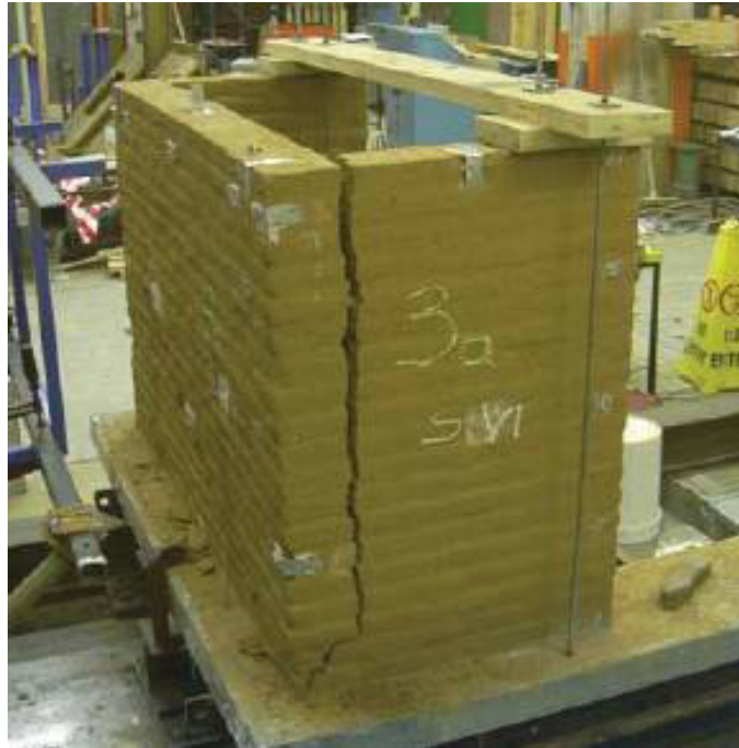
Figure 2.15: Vertical corner cracking of unreinforced u-shaped adobe wall testing at UTS, Sydney (Dowling 2006).
