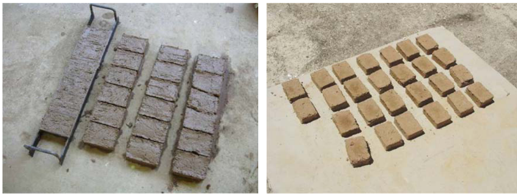
Figure 6.2: Making adobe bricks by mould.
