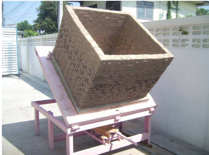
Figure 7.4: Tilt testing of a square adobe model.
