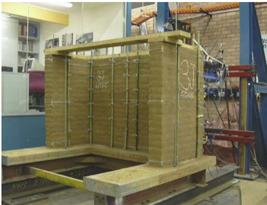
Figure 2.16 Preparation of reinforced u-shaped adobe wall unit at UTS (Dowling 2006).
