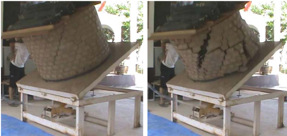
Figure 7.9: The failure modes of the circular specimens when tilted further.
