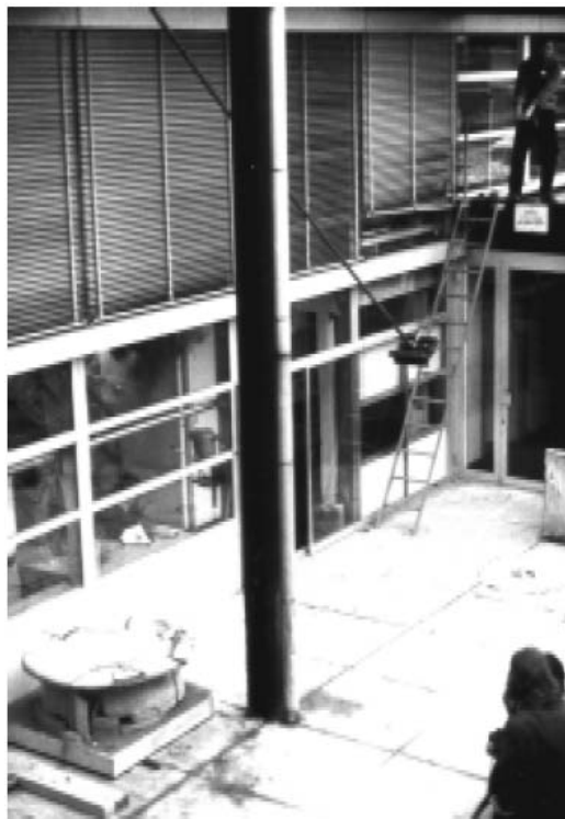
Figure 2.27: Simulation of seismic shocks (Minke 2000).
