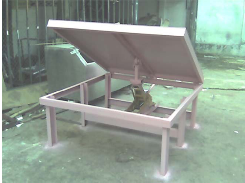
Figure 7.3: Construction of the tilt table.
