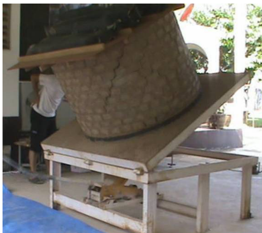
(3) Another cracking appeared.
