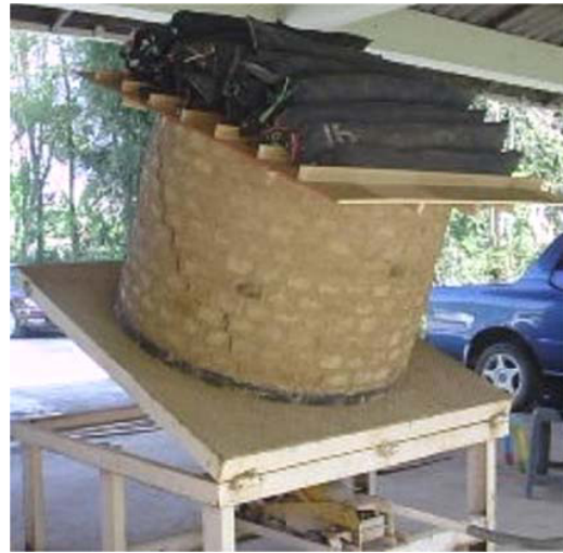
(2) The first cracking appeared.
