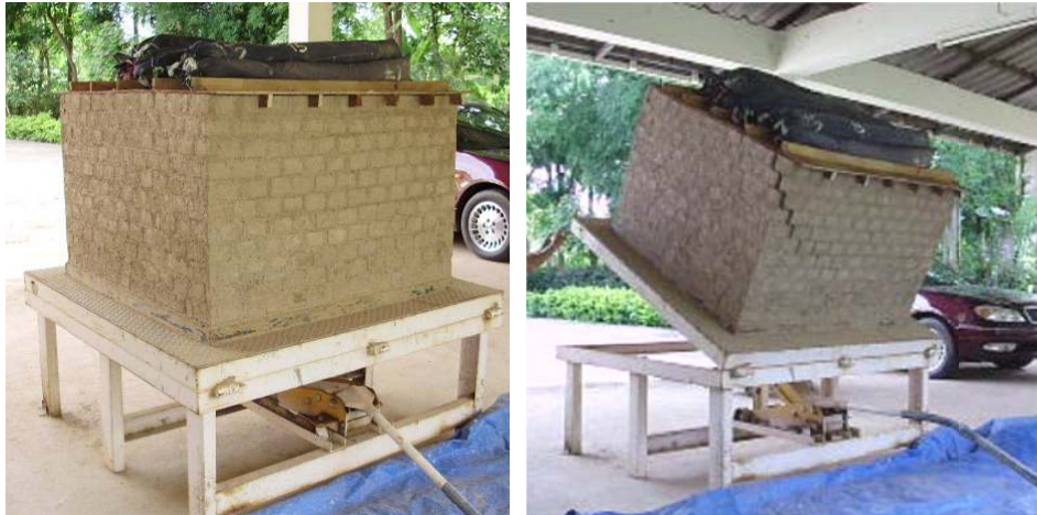
Figure 7.6: Tilting the square specimen and first crack appearing at 20 degrees.
