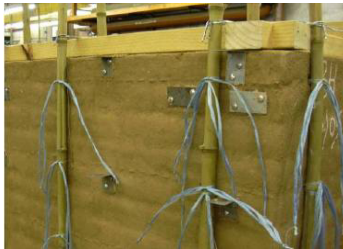
Figure 2.17: Detail of reinforcement of model adobe house at UTS (Dowling 2006).
