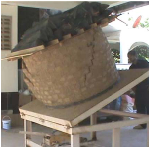
(3) Cracking from another side.
