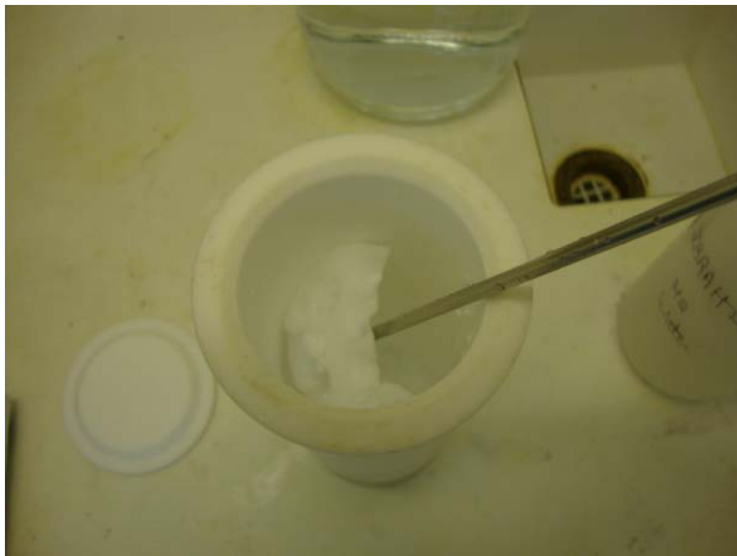
Figure 3.11. Teflon cell used for hydrothermal treatment.
