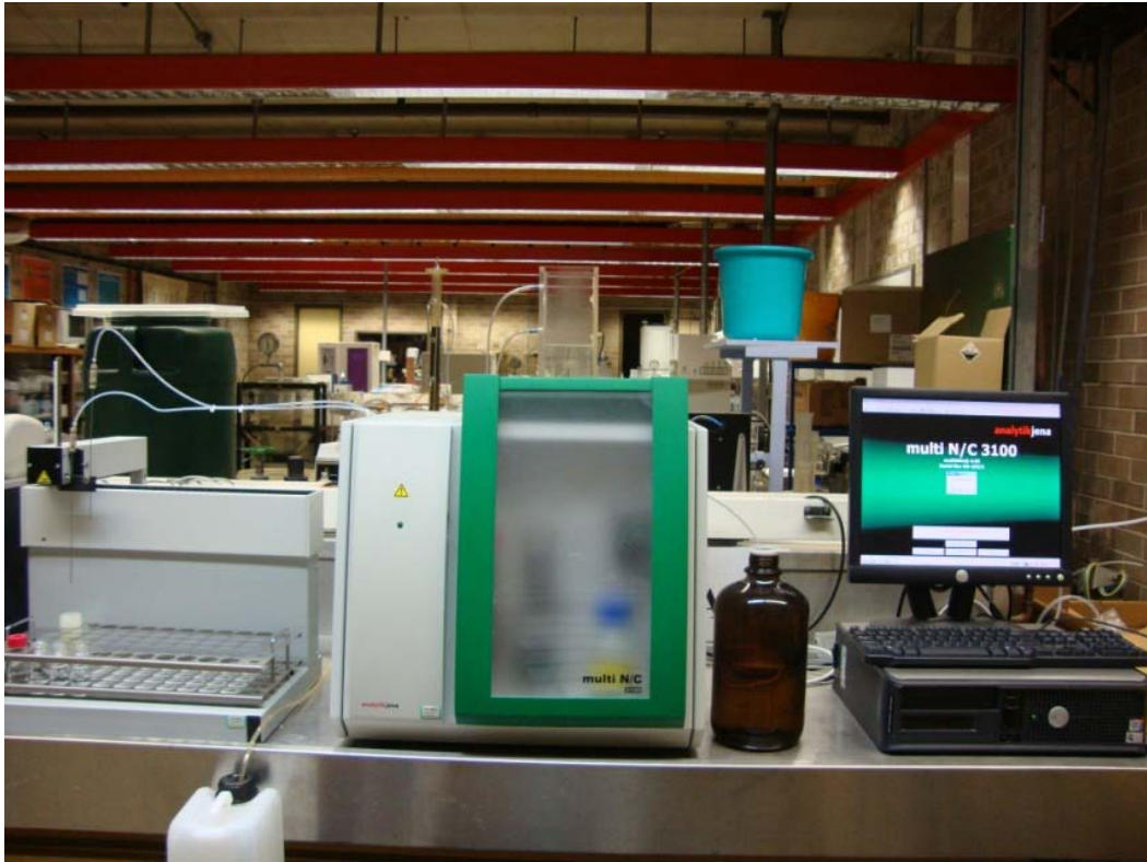
Figure 3.14. Multi N/C 3100 DOC analyser with autosampler.
