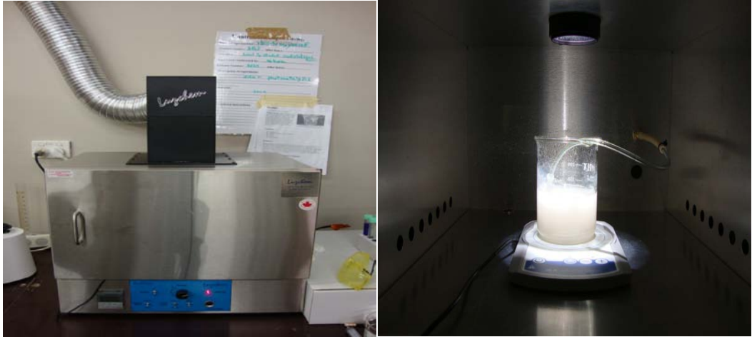
Figure 3.6. Solar simulator outside (left) and inside (right).
