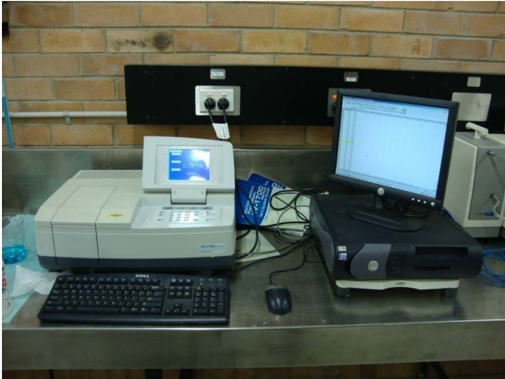
Figure 3.12. Shimadzu UV-1700 spectrophotometer.
