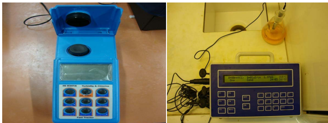
Figure 3.9. Hach HI 93414 turbidity and chlorine meter (left) and TPS pH meter (right).
