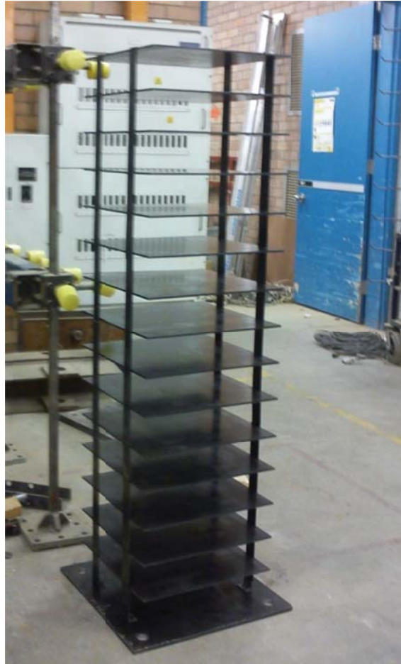
Figure 4.8: Completed structural model
