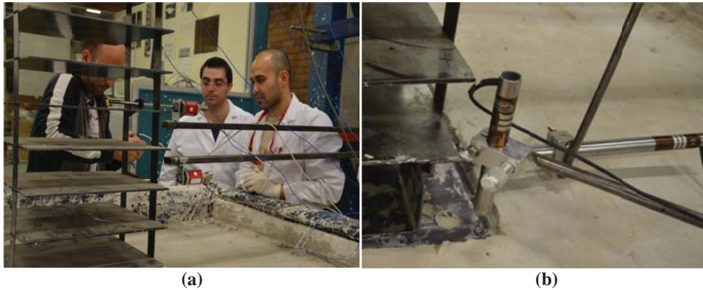
Figure 4.43: (a) Installing the displacement transducers on the structural model; (b) vertical displacement transducer installed at the level of the base plate
