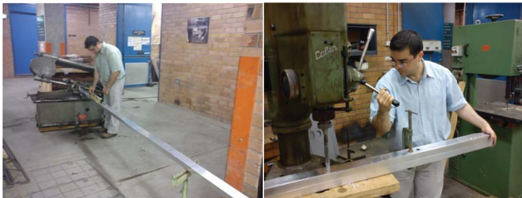
Figure 4.15: Cutting and drilling aluminium sections at the UTS structures laboratory
