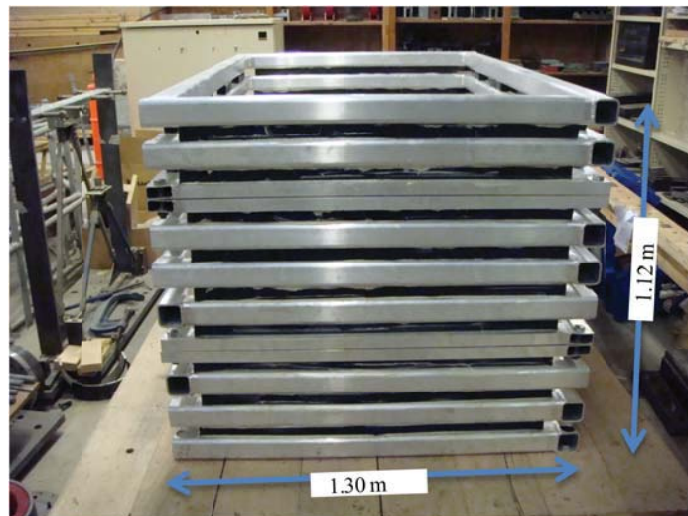
Figure 4.19: Laminar soil container view after completion of the walls
