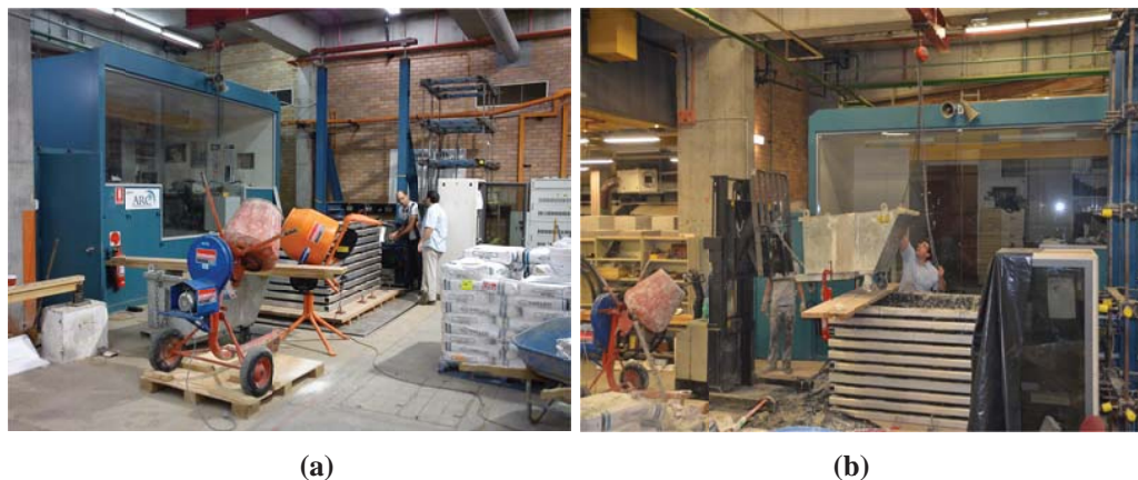
Figure 4.40: (a) Placing the mix components and mixer near the shaking table; (b) producing and placing the soil mix into the soil container
