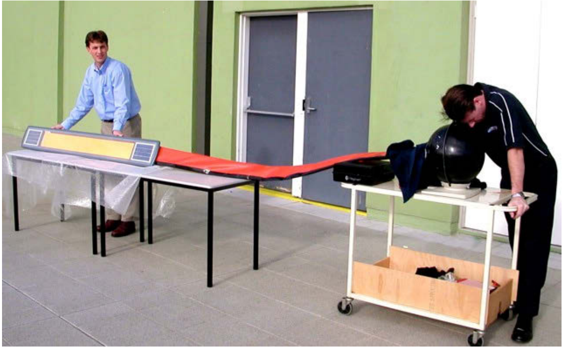
Figure 3.24 Using an integrating sphere (on the right) for the visual colour assessment of the light output from a hybrid SCATS system. The collector stack on the left has two small solar cell arrays that power blue LED's in the luminaire. The twin light guides are protected by an orange plastic sheath.
