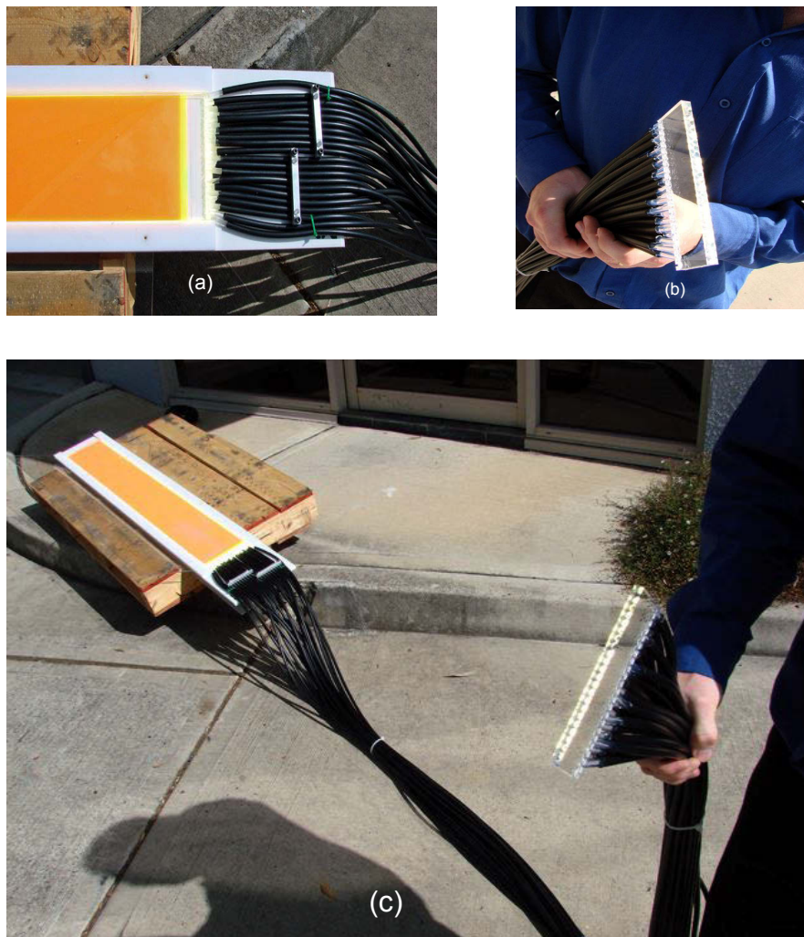
Figure 4.3 (a) Three-layer stack of fluorescent sheets connected via a coupler/mixer to 21 optical fibres. (b) The ends of the fibres are bonded to a luminaire. (c) Overview of the system.
