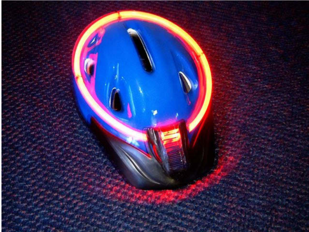
Figure 5.18 Bicycle helmet using LED's and TRIMM doped side-scattering optical fibre. Note the even brightness achieved by using a LED at each end of the fibre.
