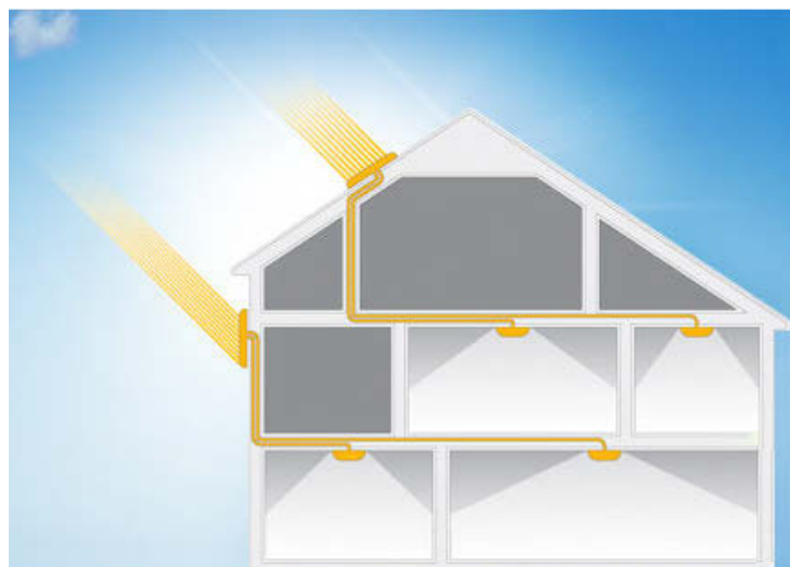
Figure 1.2 Schematic of a luminescent solar collector capturing sunlight and coupling the light into optical fibres that distribute the light throughout a building.
