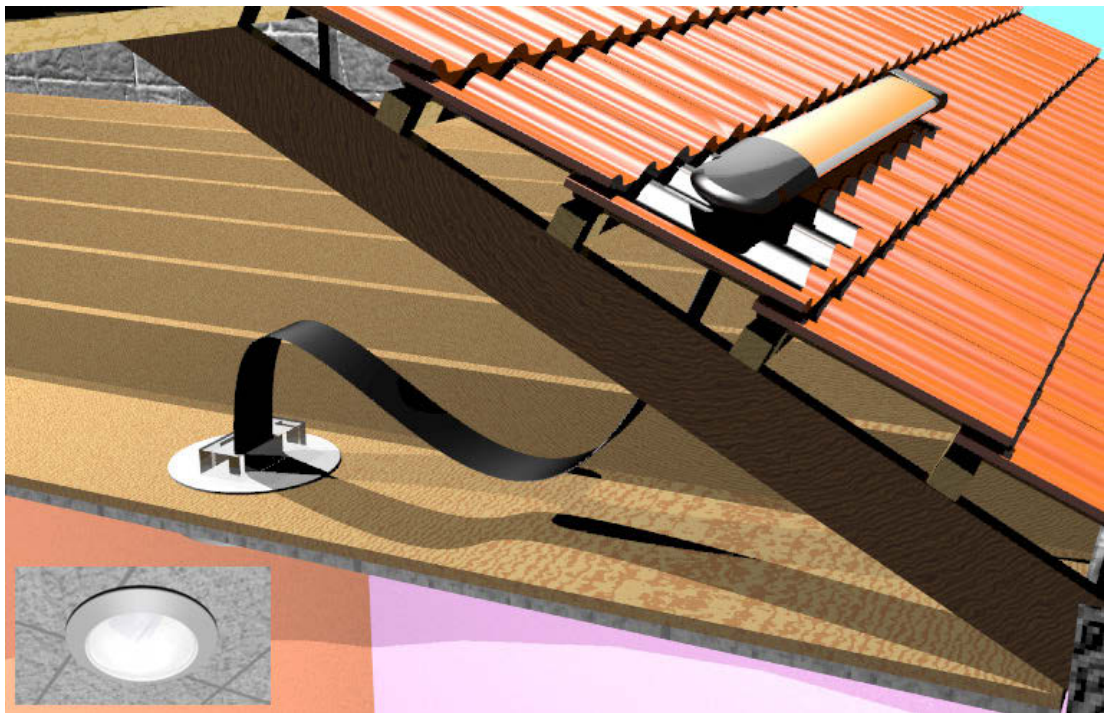
Figure 3.15 The final form of the SCATS LSC system with a three colour fluorescent stack on the roof connected by an optical conduit made from thin, flexible PMMA, connected to a luminaire.
