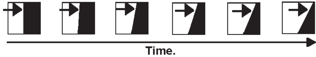
Figure 2.2: Convective mixing of a granular material.
