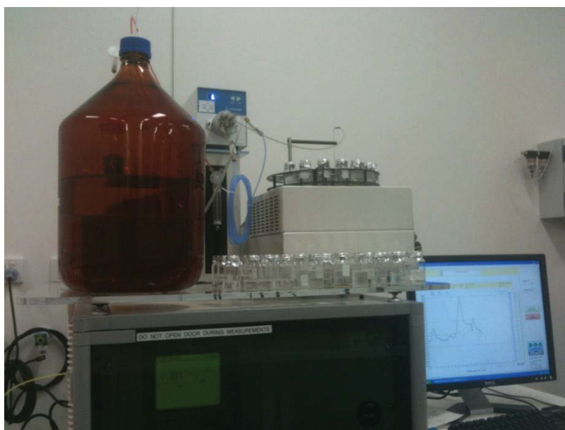
Figure 3.5 DOC-LABOR Liquid Chromatography-Organic Carbon Detector.
