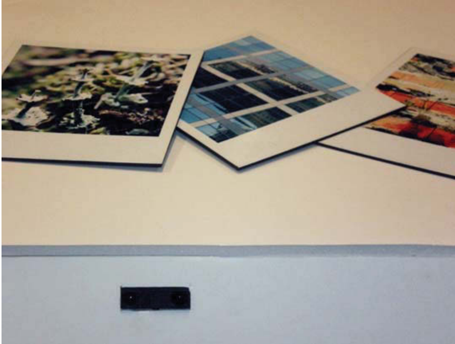
Figure 9. Proximity sensors were placed underneath the front edge of the interaction table, barely perceivable by the audience.
