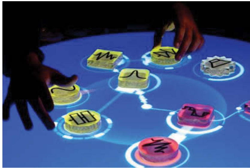
Figure 42. The reacTable and its varied-patterns objects underneath which fiducials are placed for their tracking along the surface.
